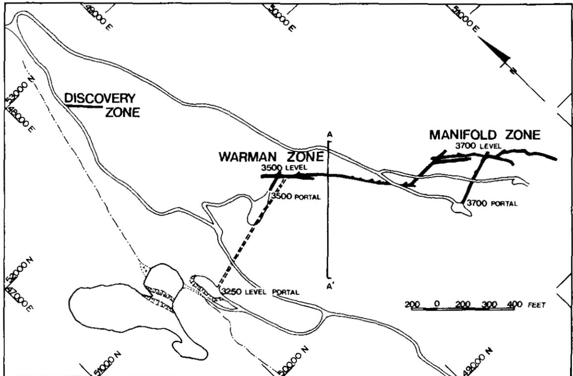
Figure 34. Generalized plan of underground haulage levels showing relative locations of three principal ore zones. A-A<sup>1</sup> is location of the cross-section of Figure 35 (modified from Dickson and McLeod, 1975).
