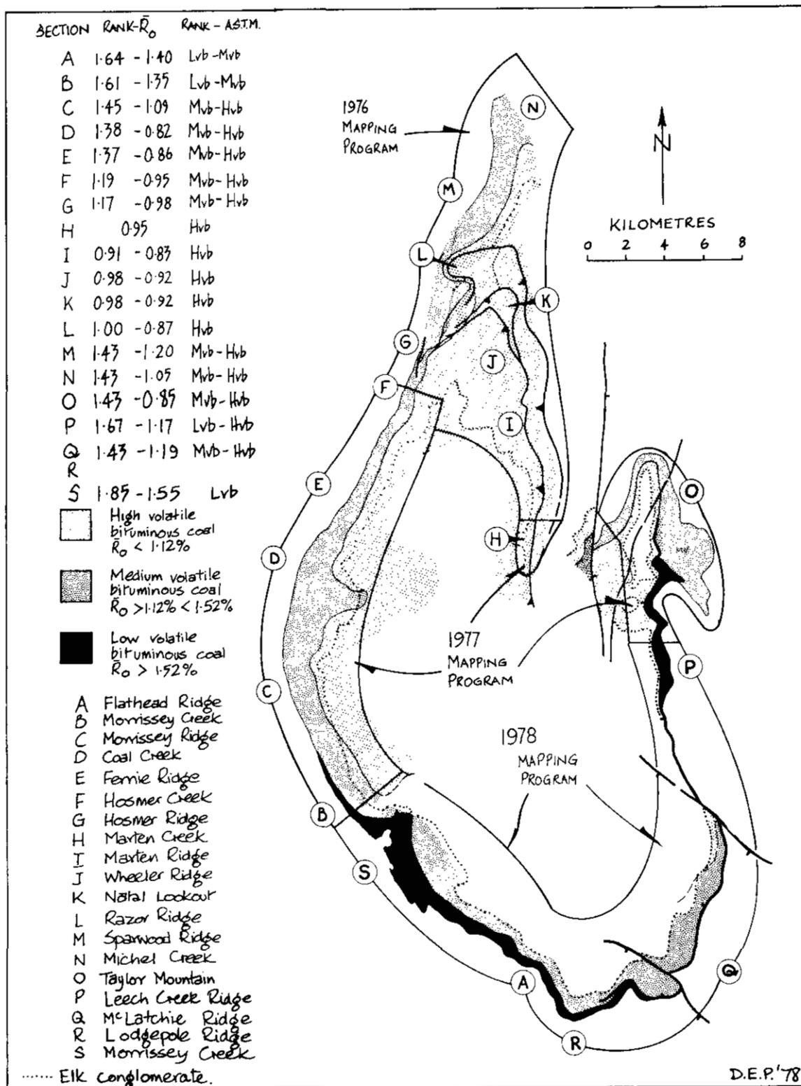
Figure 18. Distribution of low, medium, and high-volatile bituminous coals over Crownsnest Coalfield. Ranges in vitrinite reflectance data at specific locations represent coals overlying basal sandstone and underlying the Elk conglomerate.
