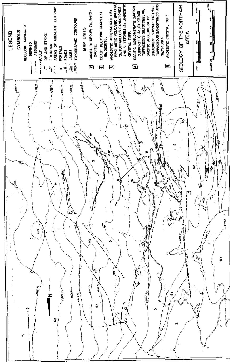
Figure 32. Detailed geological map of a part of Callaghan Creek pendant including mineral deposits of Northair Mines Ltd. Portals to the main deposits are labelled: M — Manifold zone, W — Warman zone, and D — Discovery zone. A—A1 is the location of a cross-section through the Warman zone, shown in Figure 35.
