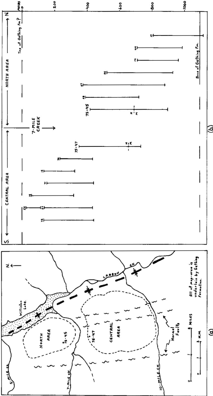
Figure 21. (a) Location map of the central and northern coal reserve areas; (b) schematic correlation chart showing the stratigraphic relationship of selected drill holes; bed 31 has been used as datum.
