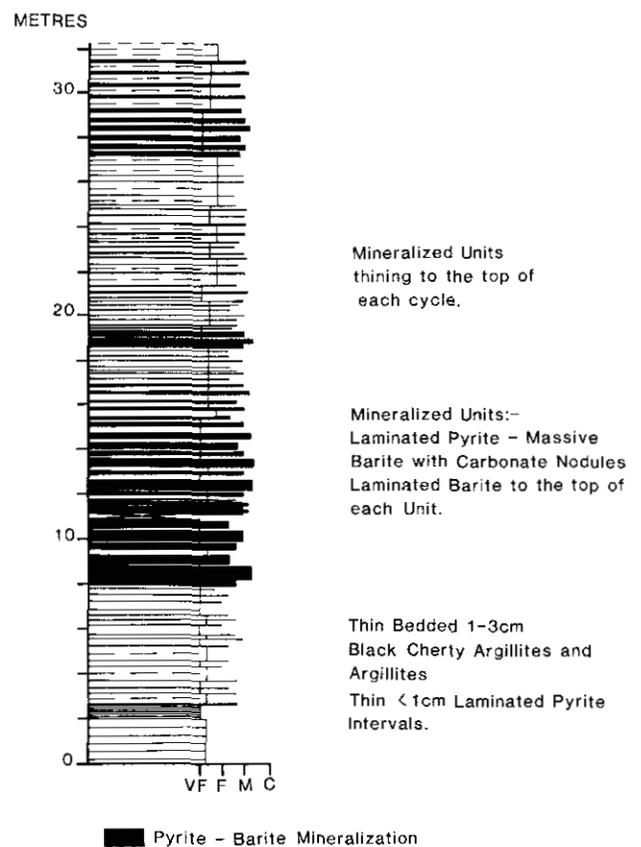
Figure 53-6. Logged section through TH mineralization from *in situ* outcrop in Driftpile Creek.
