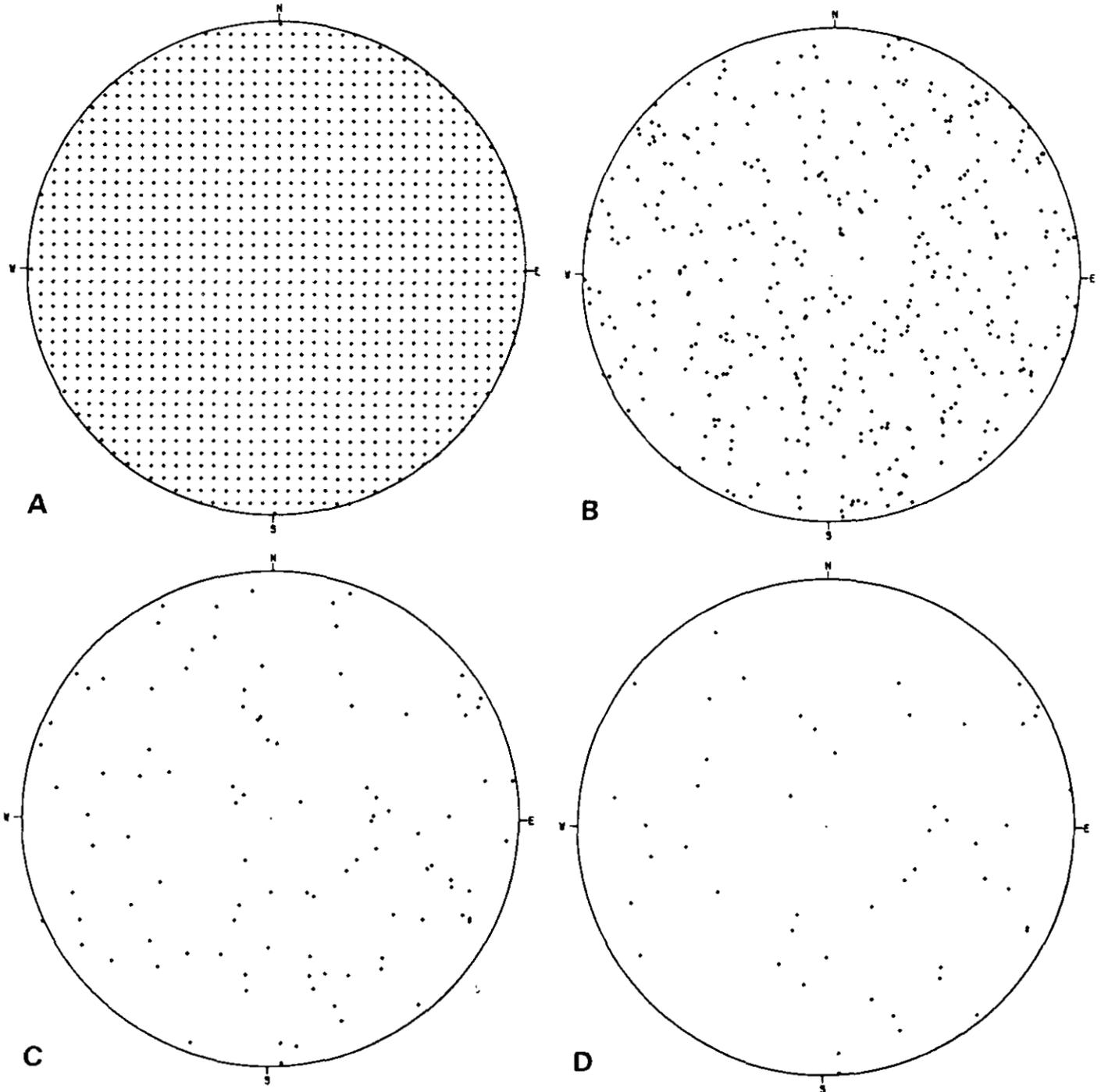
Figure 19-4. Equal area (Schmitt) projection of generated orientation data. (a) 1257 evenly distributed orientations, (b) 500 random orientations, (c) 100 random orientations, (d) 50 random orientations.
