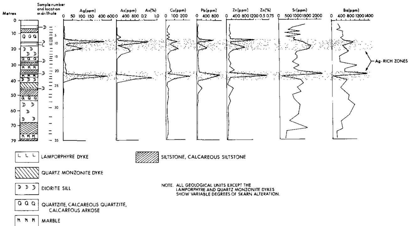
Figure 3-4. Geology and trace element geochemistry of hole SQ 84-10, Silver Queen mine.
