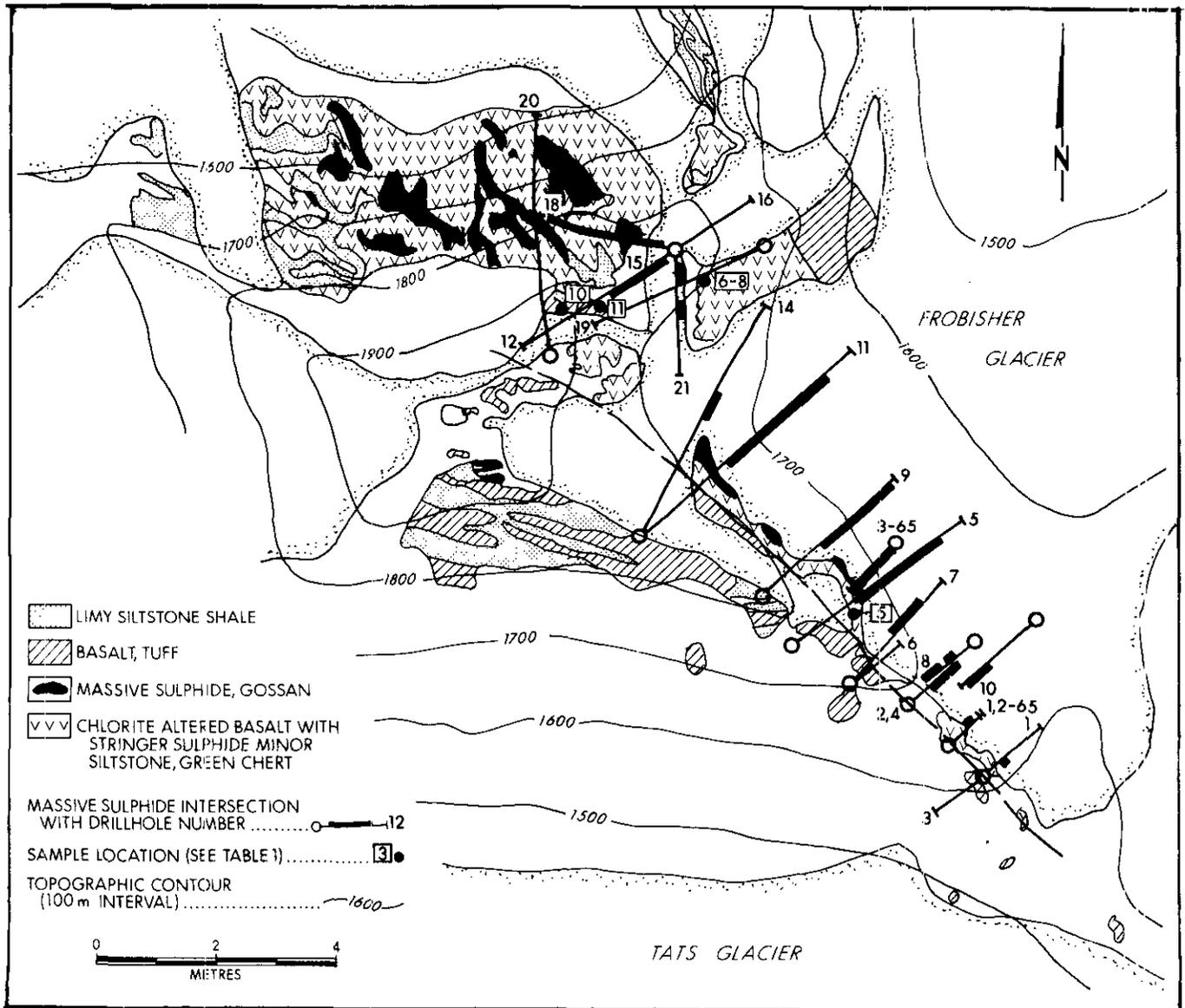
Figure 28-4. Geology, drill hole, and sample locations, Windy-Craggy deposit. Drill hole locations after company plans.
