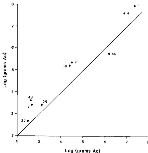
Figure 46-4. Log — log plot of total Au production versus total Ag production for Bralorne Camp. Numbers correspond to deposit numbers in Table 46-1.
