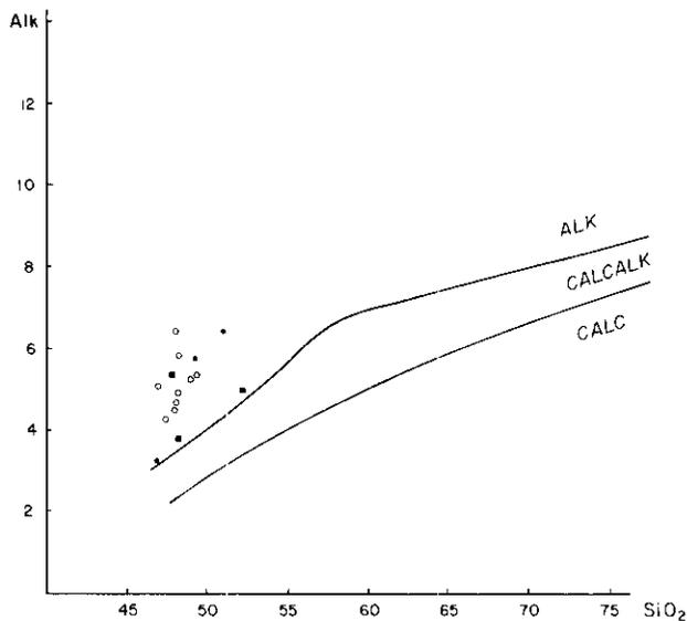
Figure 4-7. Weight per cent Alk:SiO<sub>2</sub> plot illustrates the alkaline nature of the Tillicum Mountain basalts. Boundaries from Kuno (1966), high-Al domain relabelled 'calc-alkaline' and tholeiitic domain 'calcic.'
