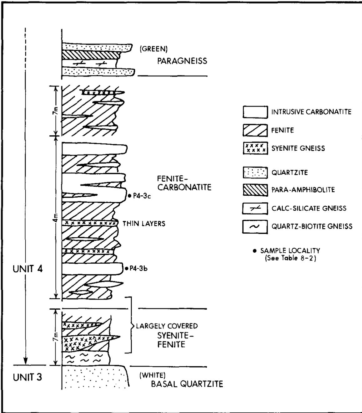
Figure 8-5. A measured section through the syenite-intrusive carbonatite-fenite zone at station H85P4 (Fig. 8-2).
