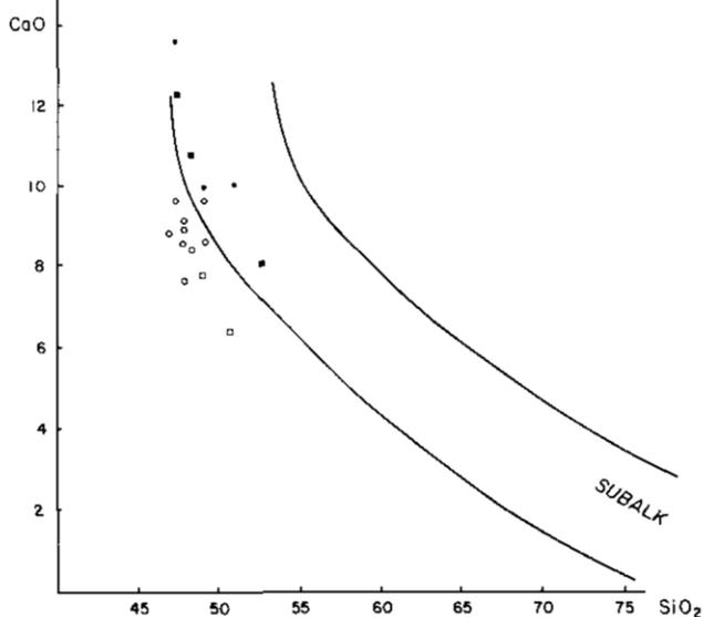
Figure 4-3. Weight percent CaO:SiO<sub>2</sub> plot shows 'unaltered' and least altered samples in the subalkaline domain. Altered samples have lost CaO. Boundaries from de Rosen-Spence (1976).
