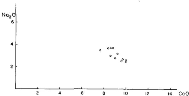
Figure 4-5. Weight percent Na<sub>2</sub>O:CaO plot shows increase in Na<sub>2</sub>O with decrease in CaO in altered samples, which indicates spilitization.
