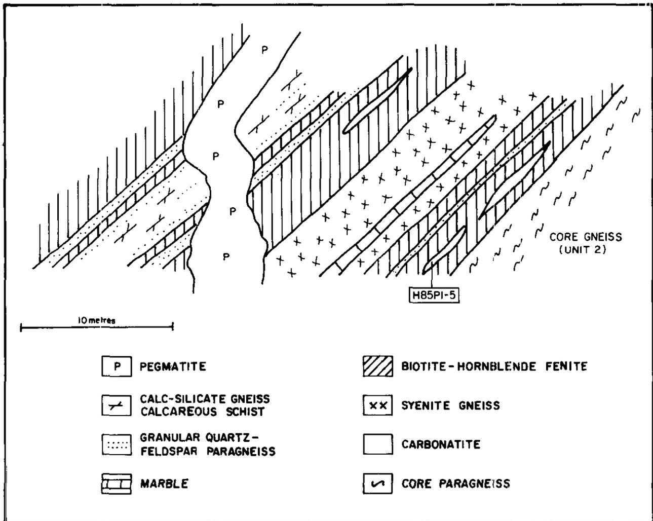
Figure 8-4. A schematic vertical section through the syenite-intrusive carbonatite-fenite zone at station H85PI (Fig. 8-2).
