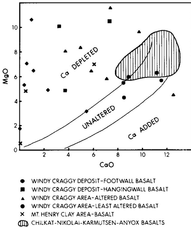
Figure 28-7. MgO versus CaO plot showing unaltered field of Spence (1985).
