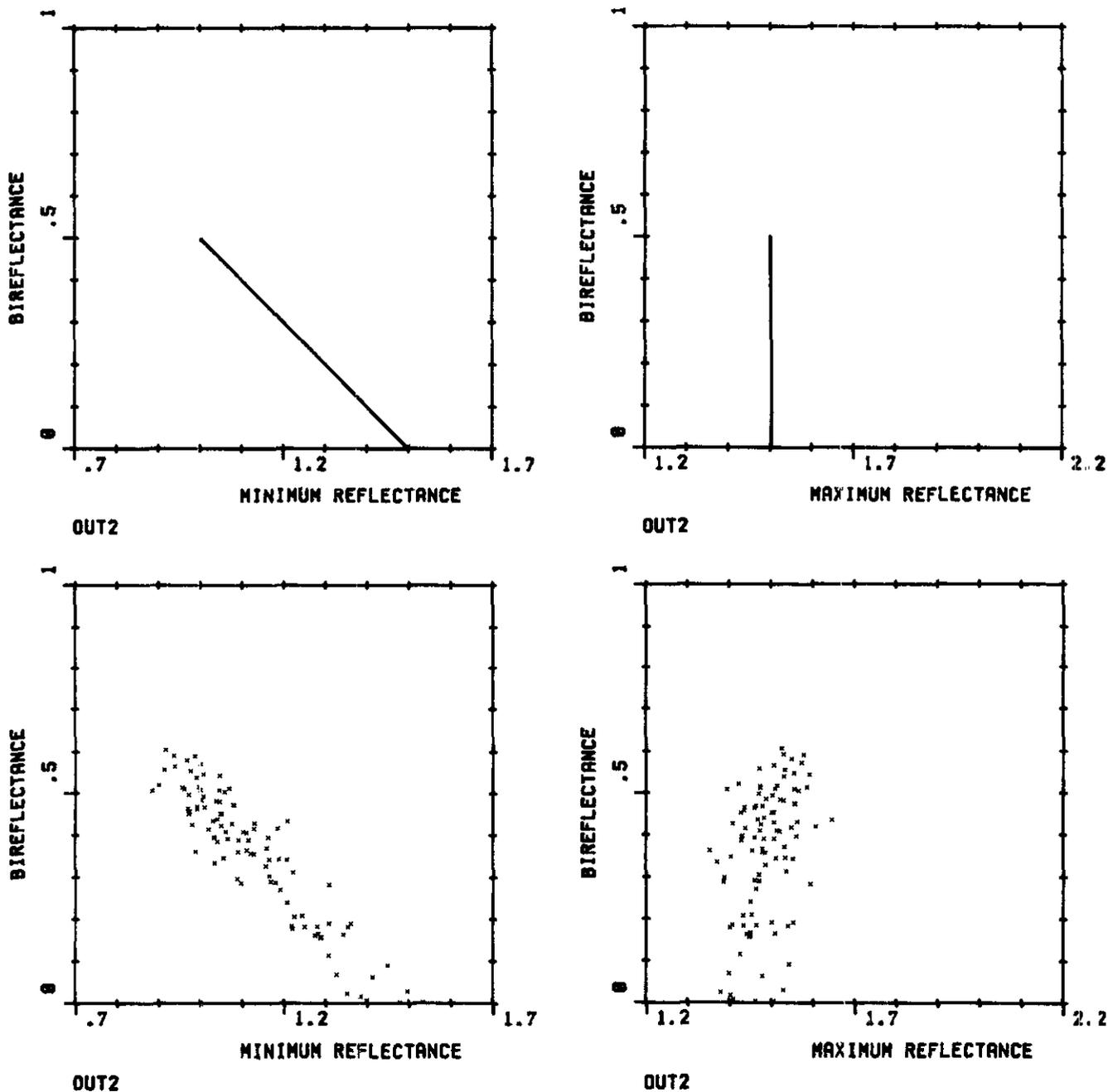
Figure 19-5. Uniaxial negative indicatrix reflectance data.  $a = 1.5\%$ ,  $b = 1.5\%$ ,  $c = 1\%$ . (a) theoretical with no variance, (b) theoretical with 0.05% standard deviation and 100 random sections.
