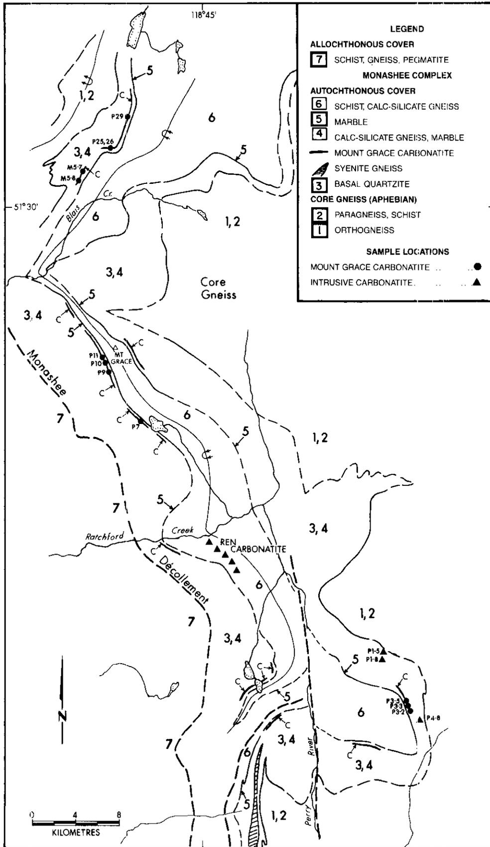
Figure 8-2. Location and structural setting of the Mount Grace carbonatite, intrusive carbonatites, and syenites in the Mount Grace-Ferry River area (geology after McMillan, 1973; Höy, 1979; Journeay, 1982). Sample locations and sites referred to in text are shown.
