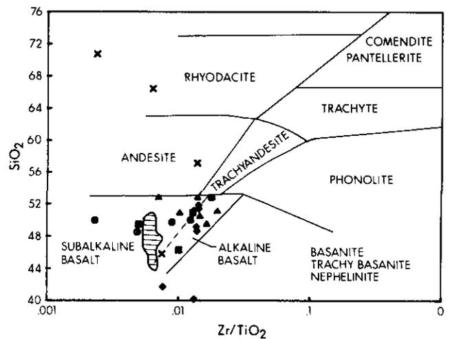
Figure 28-10. SiO<sub>2</sub> versus Zr/TiO<sub>2</sub> plot showing alkalic and subalkalic fields and rock type classification of Floyd and Winchester (1978). See Figure 28-7 for explanation of symbols.
