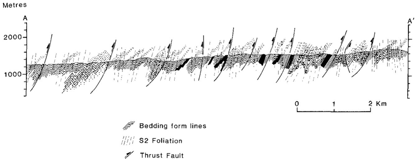
Figure 53-5. Structural section through the Driftpile Fold and Thrust Belt. Silurian siltstone is stippled.
