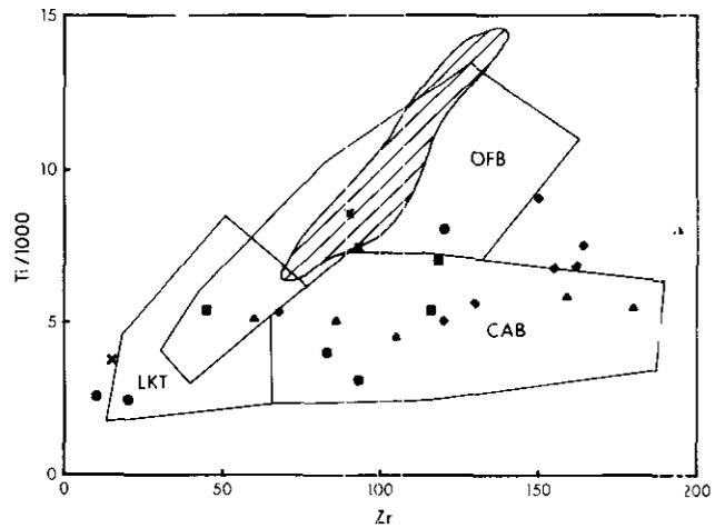
Figure 28-14. Ti/1000 versus Zr plot showing ocean floor basalt (OFB), low-K tholeiite (LKT), and calc-alkaline basalt (CAB) fields of Pearce and Cann (1973). See Figure 28-7 for explanation of symbols.
