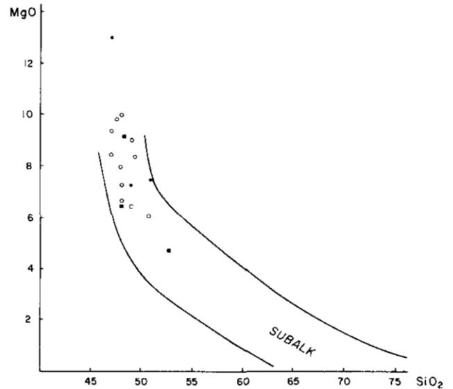
Figure 4-2. Weight percent MgO:SiO<sub>2</sub> plot. All Tillicum Mountain basalts plot in the subalkaline domain. Sample with highest MgO is a pyroxenite. Boundaries from de Rosen-Spence (1976).
