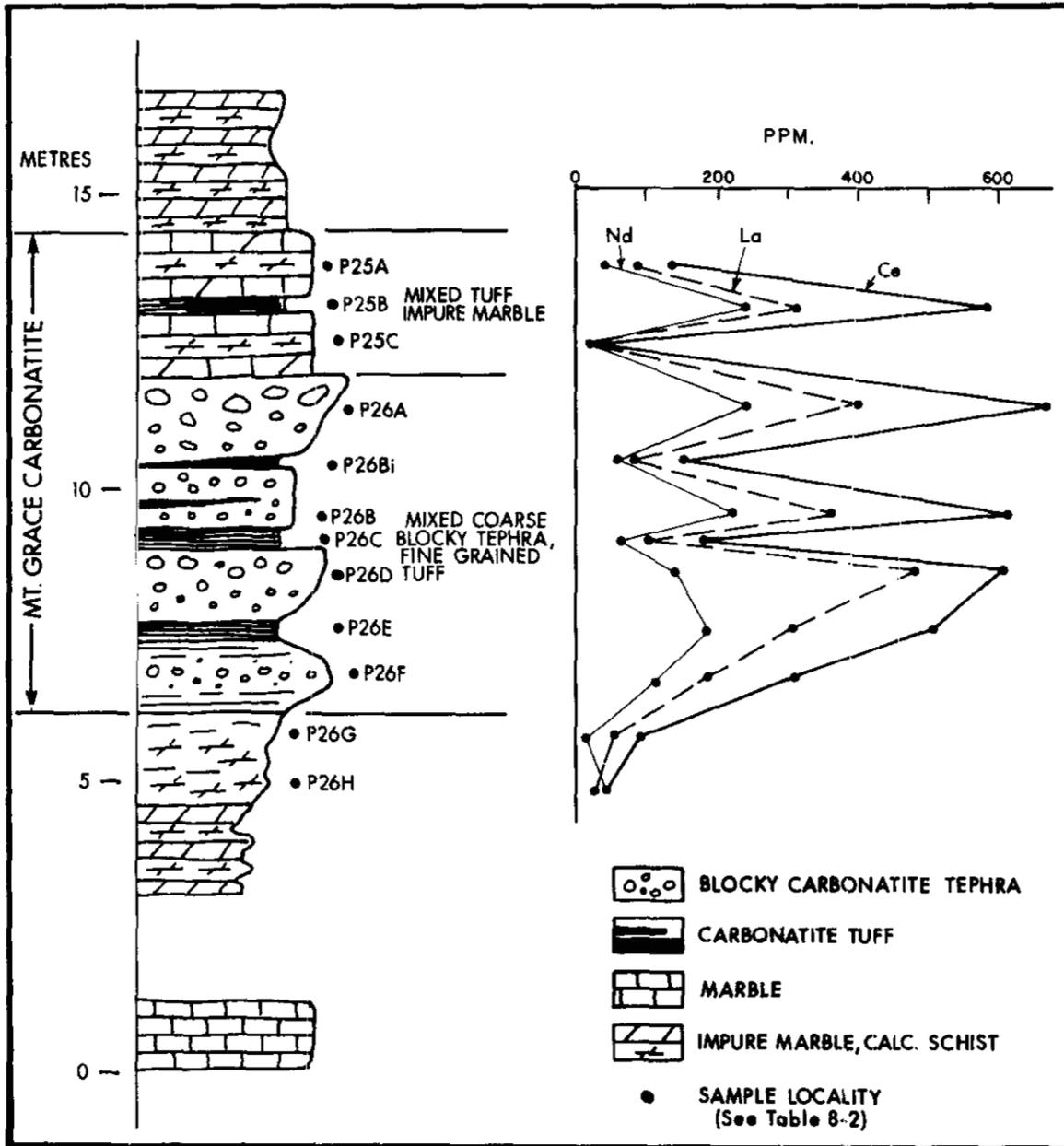
Figure 8-7. Detailed section of the Mount Grace carbonatite, Blais Creek (stations H85P25 and H85P26), showing La, Ce, and Nd values of selected samples.
