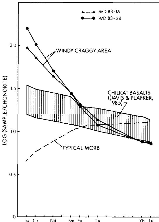
Figure 28-15. Chondrite normalized rare earth plot for two samples from the Windy-Craggy area. Also shown for comparison is the range of values for basalts from the Chilkat Peninsula, Taku terrane (Davis and Plafker, 1985), and a typical sample of MORB.
