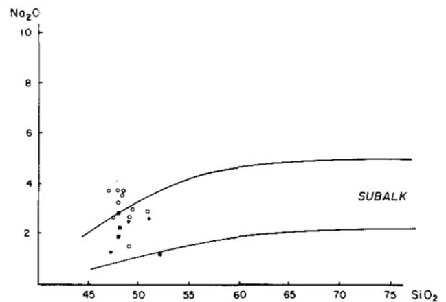
Figure 4-4. Weight percent Na<sub>2</sub>O:SiO<sub>2</sub> plot shows 'unaltered' and least altered samples in the subalkaline domain. Several altered samples have gained Na<sub>2</sub>O. Boundaries from de Rosen-Spence (1976).
