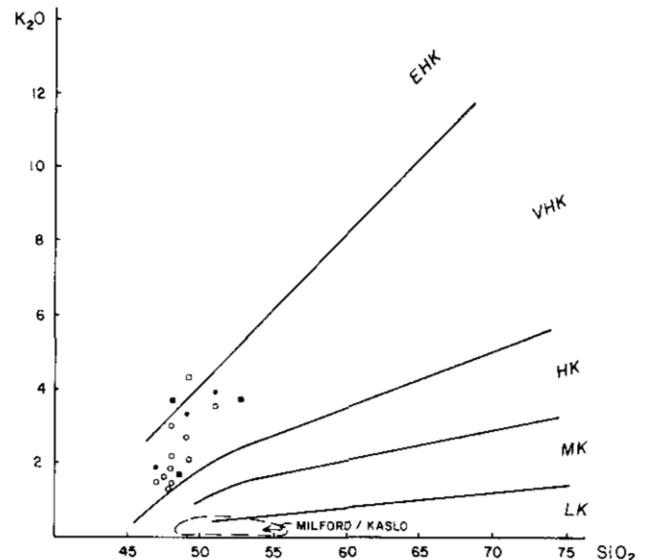
Figure 4-6. Weight percent plot demonstrates the consistently very high K<sub>2</sub>O content of the Tillicum Mountain basalts. Low (LK), medium (MK), and high (HK) K<sub>2</sub>O domains from Gill (1981); very high (VHK) and extreme high (EHK) K<sub>2</sub>O domains from Spence (1985). Note the Milford-Kaslo Groups volcanic rocks plot in the low K<sub>2</sub>O (LK) field.
