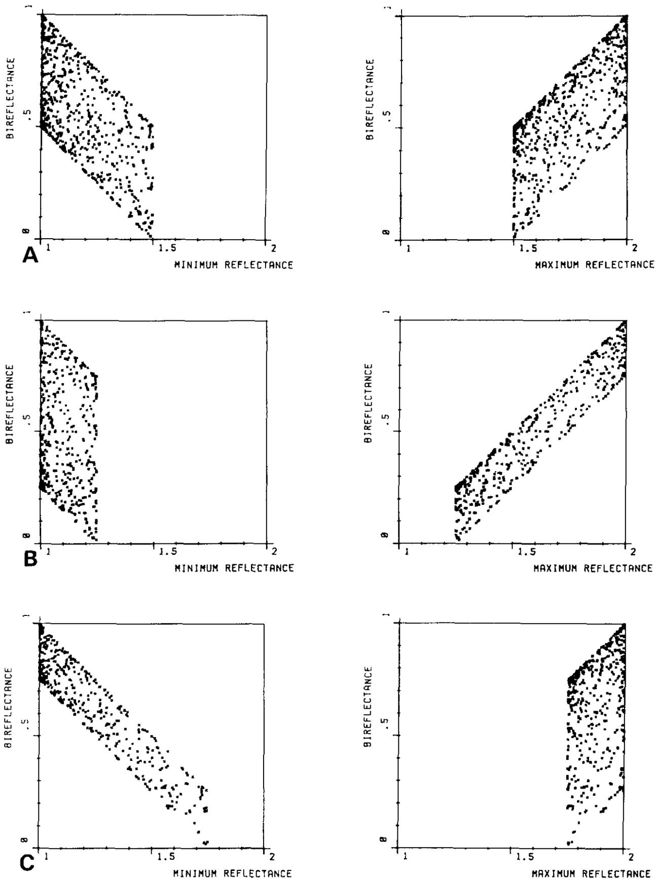
Figure 19-6. Cross-plot displays of three reflectance indicatrixes generated with randomly oriented data populations of 500 points. (a)  $a = 1.5$ ,  $b = 2$ ,  $c = 1$ , biaxial, standard deviation = 0; (b)  $a = 1.25$ ,  $b = 2$ ,  $c = 1$ , biaxial (+), standard deviation = 0; (c)  $a = 1.75$ ,  $b = 2$ ,  $c = 1$ , biaxial (-), standard deviation = 0.
