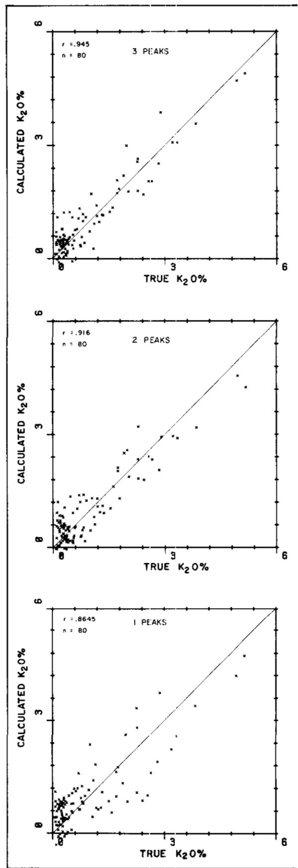
Figure 20-11. Examples of predictive regression equations for K<sub>2</sub>O content based on up to three points on the diffractograms.
