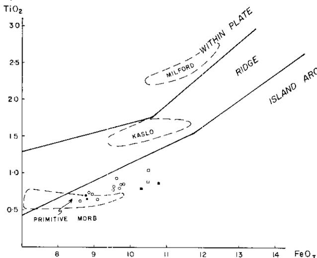
Figure 4-8. Weight per cent TiO<sub>2</sub>:FeO<sub>7</sub> plot designed for basalts with SiO<sub>2</sub> between 48 and 50.5 per cent. The Tillicum Mountain basalts are distinctly arc-type; Milford and Kaslo Group volcanic rocks plot in the within-plate and ridge domains in keeping with their setting in the Slide Mountain Terrane.
