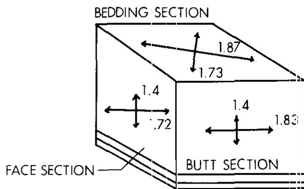
Figure 19-3. Schematic representation of the reflectance readings obtained from sample BR-U.
