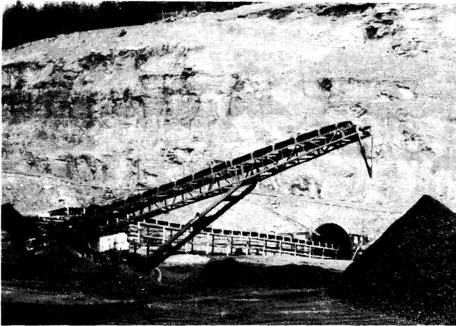
Plate 22. Underground mine entrance at Quinsam, Pit 2N. A conveyor belt transports the mined coal to the surface via this portal.
