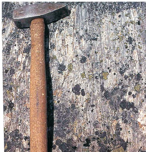
Photo 6. Strongly flattened quartz clast conglomerate, probably the “transitional unit”.
