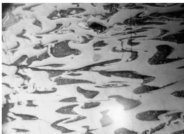
Photo 7. Deformation of semifusinite; field of view 0.25 mm.
