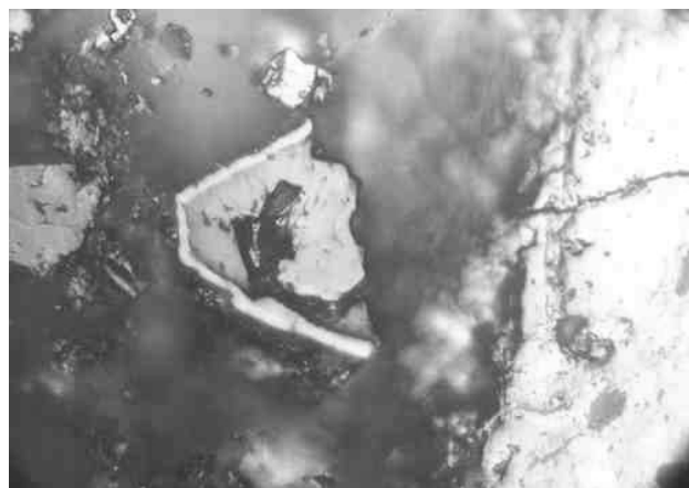
Photo 3. High reflecting rim to vitrinite grain; field of view 0.25 mm.
