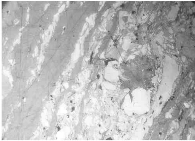
Photo 2. Calcite in 1980-69 occurring as small blebs in desmocolinite; field of view 0.25 mm.
