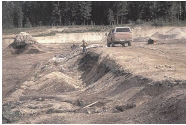
Photo 1. View of the Red Lake mining operation. Upper carbon-rich unit ( Muc ) containing leonardite is exposed within the bench in the central portion of the photo.
