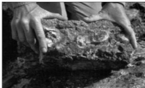
Figure 7. Typical chunk of the Yurso vein, rusty-stained quartz with pyrite, arsenopyrite, tetrahedrite and stibnite.
