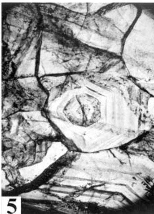
Photo 5. Growth zones in skarn garnet. Zones are defined by large, irregular-shaped type I fluid inclusions. Sample GR01-31. Transmitted plane light. Long field of view is 2.63 mm.
