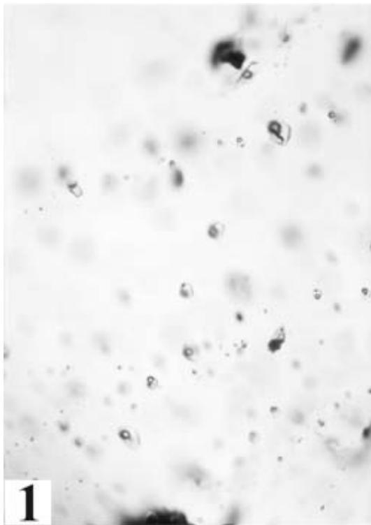
Photo 1. Fracture planes in a Mo-bearing quartz vein from the porphyry defined by secondary type III halite-bearing fluid inclusions, each containing a cubic-shaped, opaque daughter mineral. Sample GR01-60. Transmitted plane light. Long field of view is 0.64 mm.
