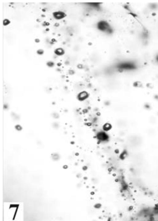
Photo 7. Fracture planes in quartz from a Mo-bearing quartz porphyry vein in the Glover Stock. Planes are defined by secondary vapour-rich type II fluid inclusions only. Sample GR01-60. Transmitted plane light. Long field of view is 0.64 mm.
