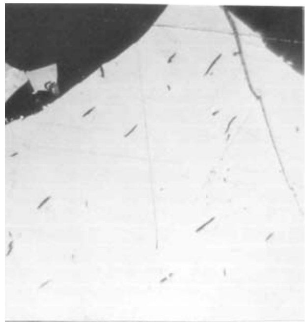
Photo 1. Pseudo vitrinite in Gething coal showing elliptical cavities. Width of photo approximately 0.2 mm.
