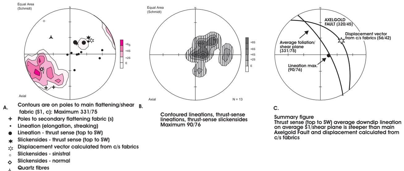
Figure 8. Structures on and near the Axelgold property.
