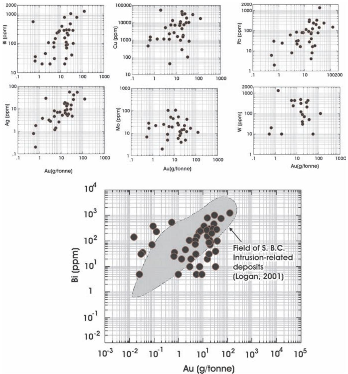
Figure 5. Geochemical correlation diagrams: Hawk vein samples: plotted vs. Au. Data from Redcorp Ventures Ltd.; Eco-Tech Laboratories analysis.
