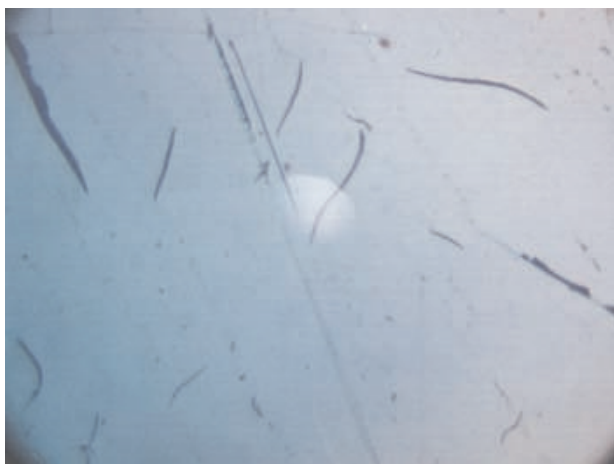
Photo 4. Pseudovitrinite with multiple orientations of slits.
