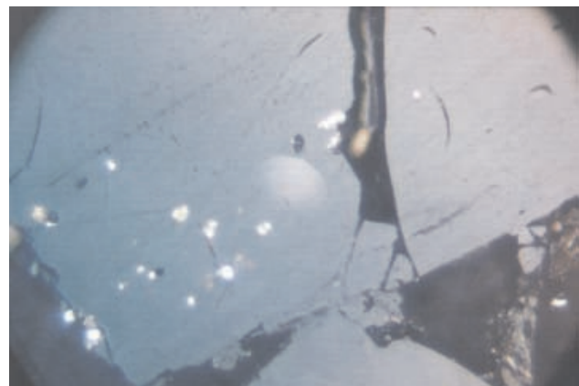
Photo 3. Pyrite in pseudovitrinite grains.
