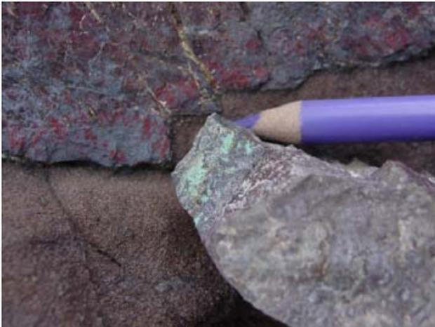
Photo 5. Copper staining on argillaceous bedding planes at the interbedded contact between marley ferruginous chert and limestone.
