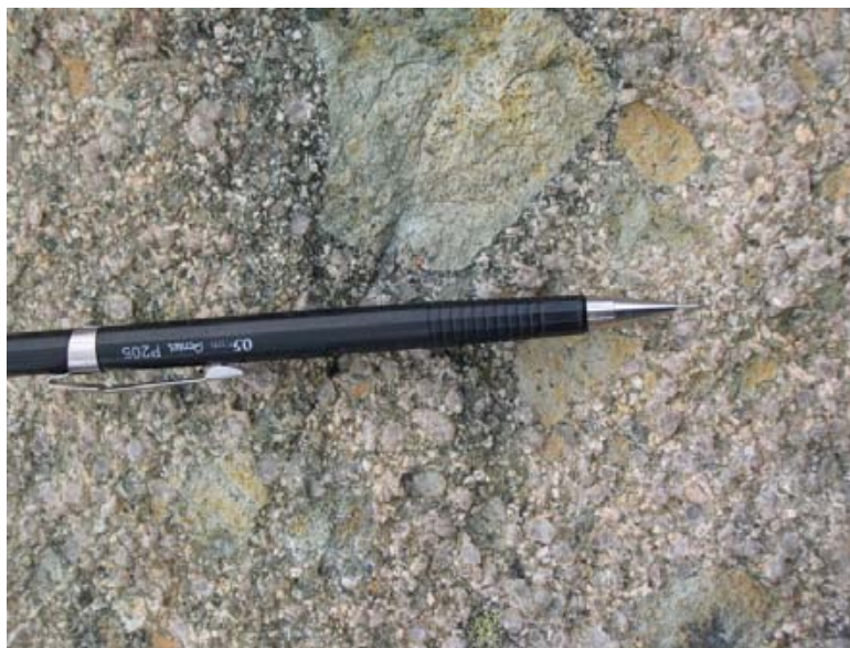
Figure 8. Very coarse-grained quartz-eye feldspathic sandstone in the Rivers Peak area. Gritty-looking regions comprise euhedral to subrounded and broken quartz and plagioclase. Rusty orange and green, more coherent splotches comprise aphanitic, mafic to intermediate volcanic clasts that occur near the base of this unit. Pencil (~8 cm) for scale.
