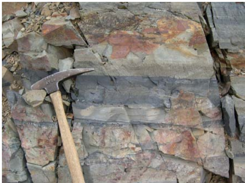
Figure 5. Tuffaceous mudstone sequence with possible syngenetic sulphide mineralization at Tesla Mountain. Rock hammer (~40 cm) for scale.
