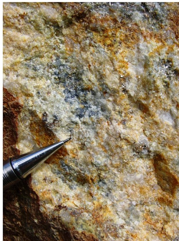
Figure 5. Blue-grey molybdenite occurs in irregular clots up to fist size at the Big Joe occurrence. Highly reflective mineral grains are pyrite and white mica.
