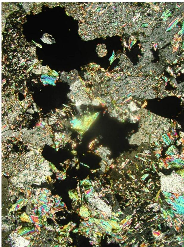
Figure 4. Photomicrograph of typical alteration assemblage in granite stock hosting molybdenite mineralization at the Big Joe. The long dimension of the photo represents approximately 4 mm and the photo was taken using cross-polarized light. Brightly coloured (high birefringence) mineral grains are white mica; opaques are mainly pyrite and minor molybdenite.
