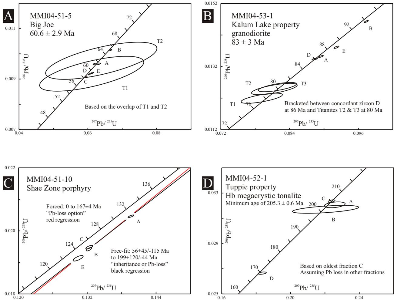
Figure 3. Concordia plots of isotopic data and interpreted ages. Data were obtained from analysis of samples from four intrusive bodies in the Kitsumkalum Lake area. See Figure 2 for locations and Table 1 for analytical data.
