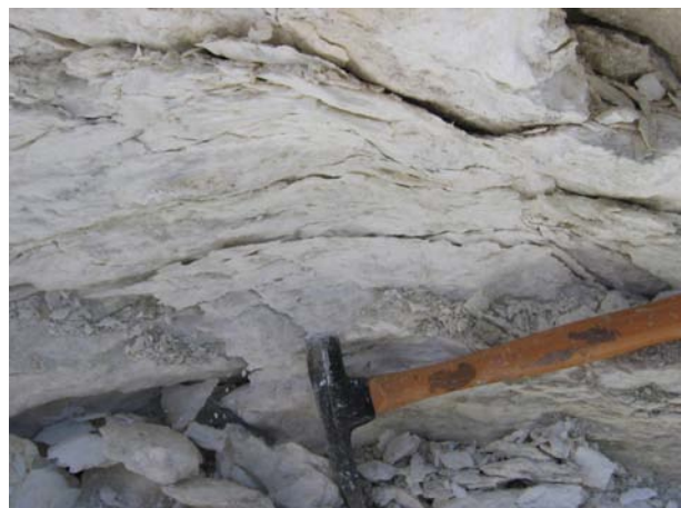
Figure 6. Strong preferential fabric and snow white colour characterizes talc-bearing zone, Bridesville, southern BC. Hammer for scale.
