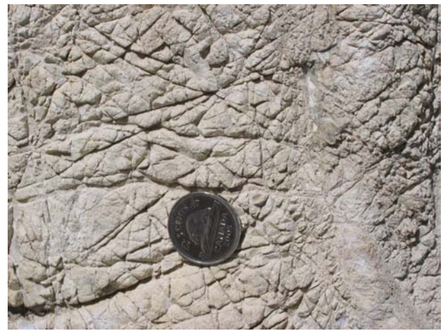
Figure 4. Weathered surface of dolostone showing nearly random fracturing, Bridesville talc-carbonate deposit, southern BC. Fracture pattern is enhanced by preferential weathering. Five-cent coin for scale.
