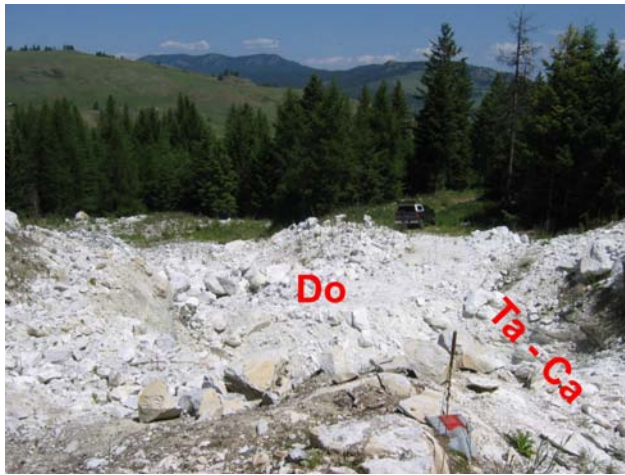
Figure 2. View of the excavation at Bridesville talc-carbonate deposit, southern BC; looking north (truck for scale). Abbreviations: Do, dolostone; Ta-Ca, talc-carbonate zone.
