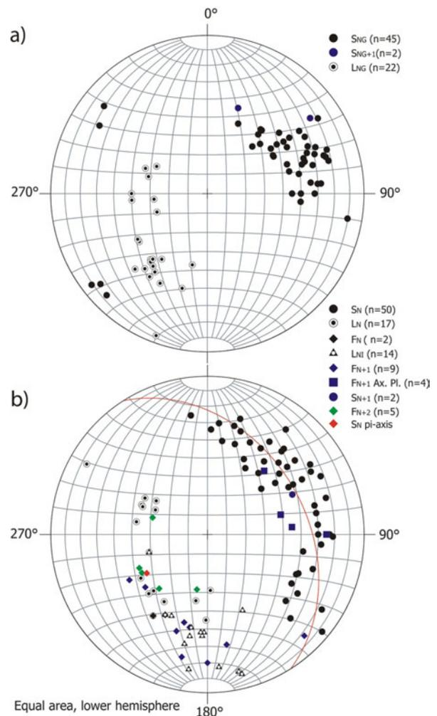
**Figure 4.** Equal-area lower-hemisphere stereonet projections of structural data from the western margin of the Naver I pluton and adjacent rocks: **a)** data from the Naver I pluton; **b)** data from rocks of the Snowshoe Group, Crooked amphibolite and Nicola Group (black phyllite unit) adjacent to the western margin of the intrusion.
