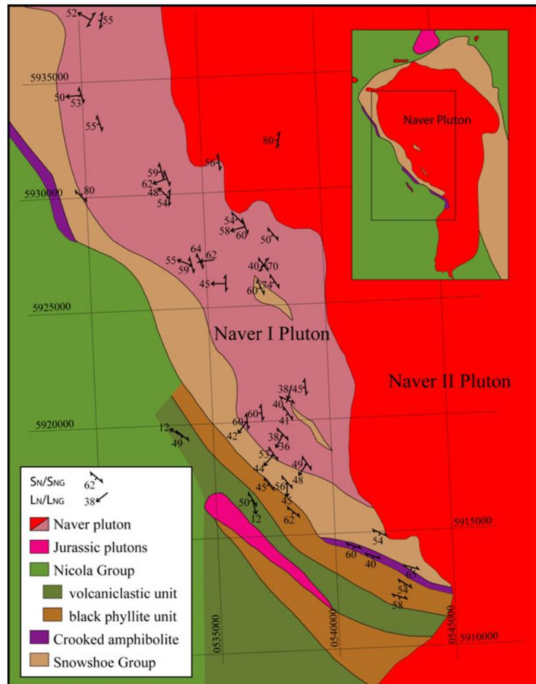
**Figure 2.** Map of the western margin of the Naver pluton, modified after Massey et al. (2005) and based on 2008 fieldwork. The inset shows the full extent of the Naver pluton and its relationship to the boundaries separating the Nicola Group, the Crooked amphibolite and the Snowshoe Group.
