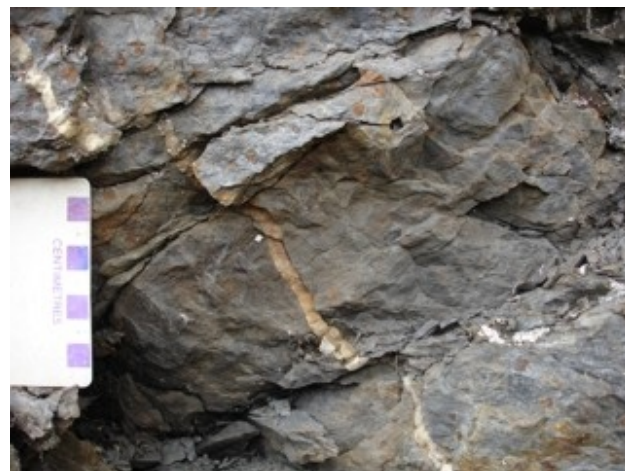
Figure 5. Typical argillite with graphitic fracture surface showing rusty weathered pyrite, Fe-Mg carbonate and a displaced and distorted quartz vein (08KAP 04-07, UTM Zone 11, 604310N, 5828487E, NAD 83).
