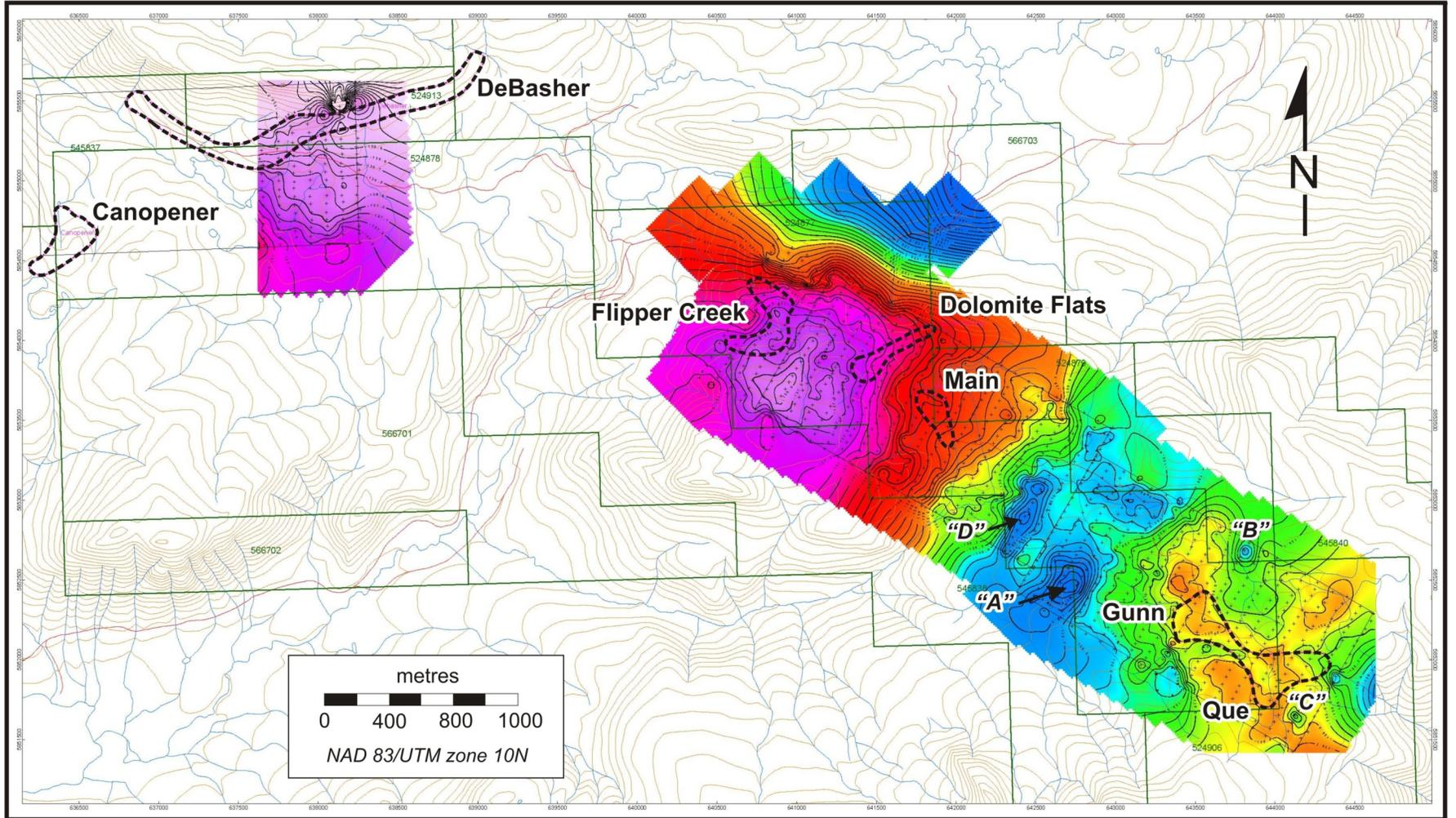
**Figure 4.** Cariboo Zinc property, east-central British Columbia, showing ground gravity contours of calculated Bouguer gravity anomalies (Luckman, 2008). Anomalies A, B, C, and D are discussed in the text.
