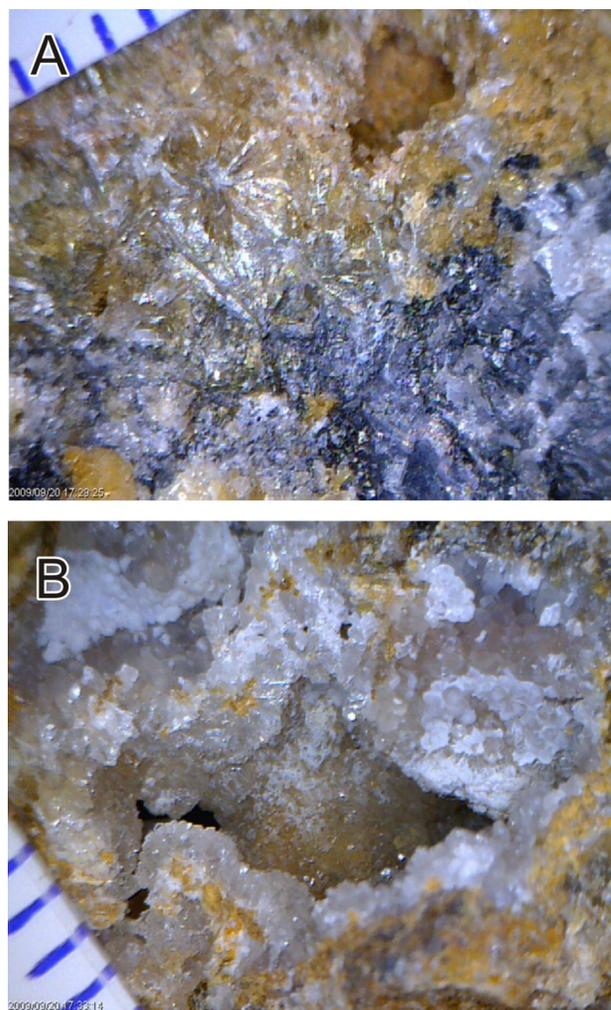
**Figure 9.** Gunn showing, Cariboo Zinc property, east-central British Columbia: **A**) white to pale grey, translucent to transparent radiating crystals, 2–3 mm in length (probably cerussite); **B**) stubby white transparent crystals (probably anglesite) lining cavities.
