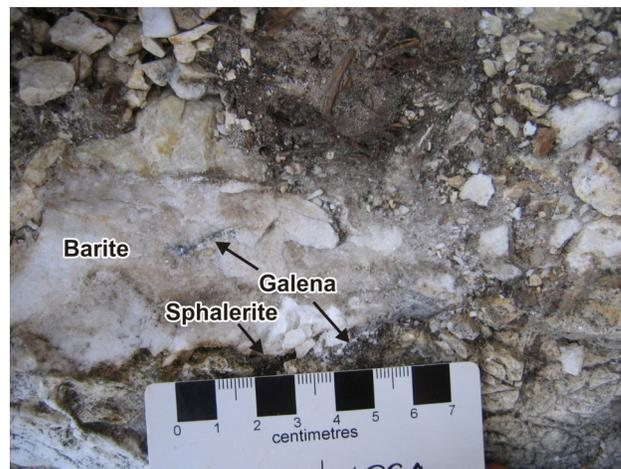
**Figure 5.** Barite vein with seams of galena at the border and in the middle of the vein, Flipper Creek prospect, Cariboo Zinc property, east-central British Columbia.
