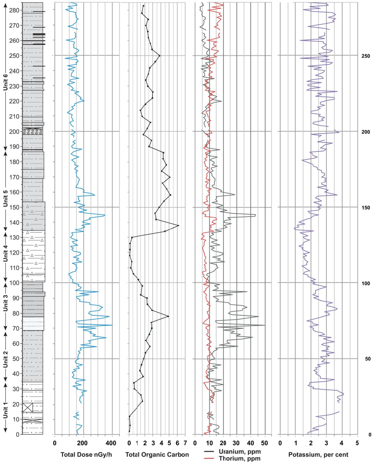
**Figure 11.** Comparison of main lithologic units of the measured Besa River Formation section with measured levels of total gamma ray counts, uranium, thorium, potassium and total organic carbon.
