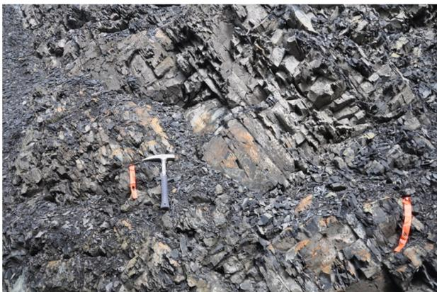
**Figure 10b.** General shot of grey to dark grey weathering siltstones of unit 3 at the 80 m level.
