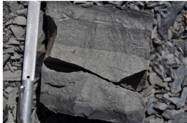
**Figure 12e.** Close-up of fresh surface across the lower sulphide horizon at the 257 m level showing the bedded nature of the pyrite mineralization and the variation in its concentration which could be attributed to settling from the water column.
