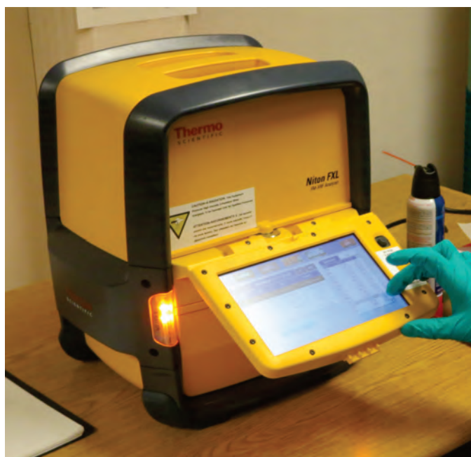
Fig. 3. The pXRF Thermo Fisher Scientific Niton FXL-950 instrument used in this study.
