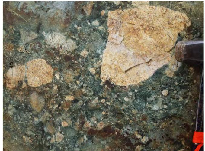
**Fig. 7.** Hazelton Group volcaniclastic unit polymictic pebble-cobble conglomerate, Billygoat bowl. The pinkish felsic intrusive clasts are texturally similar to the small plugs on top of Snippaker Ridge, which are interpreted as feeders to the volcaniclastic sequence. 381430 E, 6280469 N.
