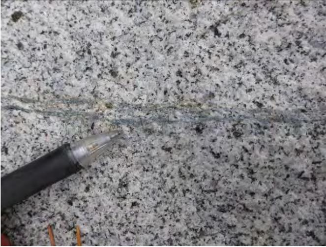
**Fig. 16.** Typical salt and pepper Pennask tonalite, here with minor grey-green fault planes lined by chlorite.
