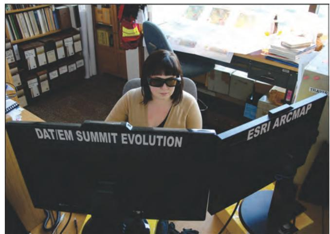
**Fig. 10.** BCGS geomorphologist mapping surficial geology on the recently acquired Summit Evolution photogrammetric 3D workstations.
