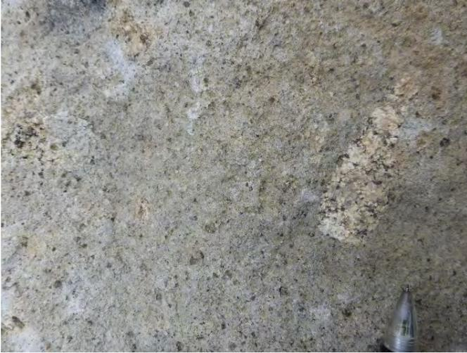
**Fig. 13.** Princeton Group. Quartz-eye, biotite-bearing rhyolite with accidental fragments of granodiorite.
