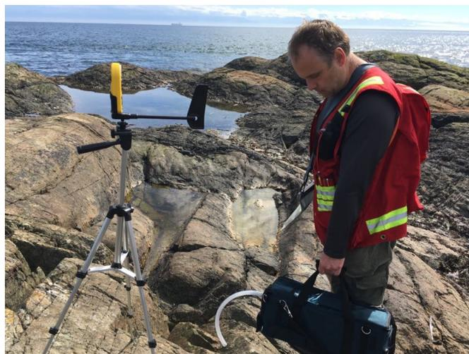
Fig. 2. Simultaneous measurement of meteorological conditions and Hg vapour concentrations in near-surface air at Harling Point, southern Vancouver Island.
