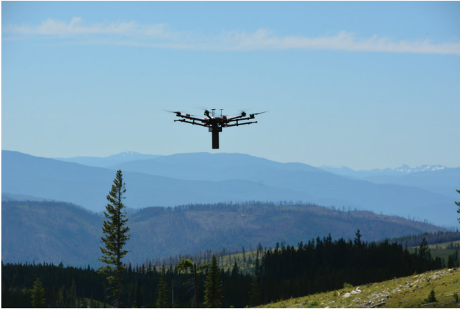
Fig. 10. Radiation Solutions Inc. RS-530 gamma-ray spectrometer, mounted to a DJI Matrice 600 Pro, completing a survey north of Merritt above tills derived from Bethsaida phase (Late Triassic) granodiorite, Guichon Creek batholith.
