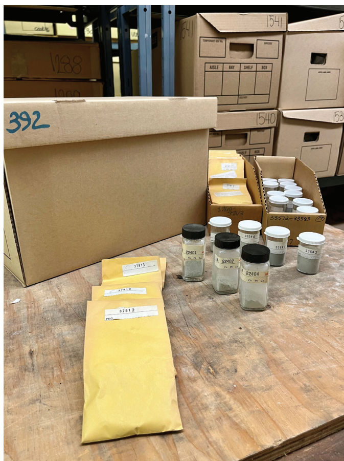
Fig. 3. Examples of pulverized rock samples (pulps) at the BCGS Sample Archive. A unique, five-digit laboratory identifier (ID) links the original sample ID, analytical, and other metadata captured in the provincial rock litho-geochemistry database. A geochemical sample catalogue captures sequences of sample IDs per tray, along with the corresponding archive box number, type of sample medium, and other sample metadata.
