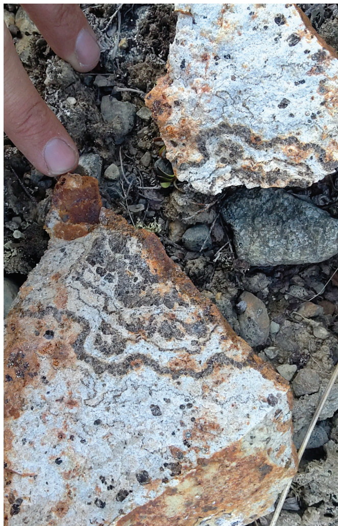
Fig. 5. Dark grey verticulate quartz veins ('brain rock') and smoky, almost black, quartz eyes in a fine-grained, aplitic matrix is the high-level, porphyritic part of the Gladys Lake body (Surprise Lake intrusive suite). Traces of molybdenite have been found in some of these veins.
