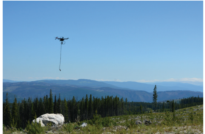
Fig. 13. DJI Matrice 600 Pro aircraft mounted with a GSMP-35U magnetometer (DRONEmag) flying from right to left at a height of about 7.5 m above ground level. See Elia et al. (2024b).
