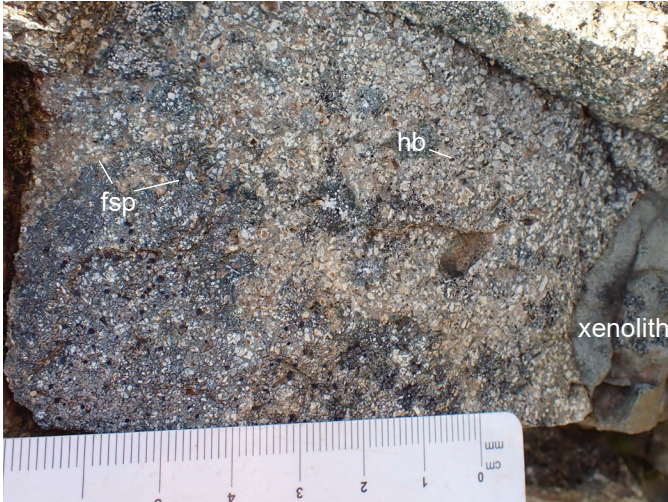
Fig. 19. Texas Creek plutonic suite monzodiorite unit (EJTdmzd) from the unnamed body 6 km northwest of the Ball Creek porphyry occurrence. Medium-grained, hornblende-feldspar porphyry crowded porphyry.
