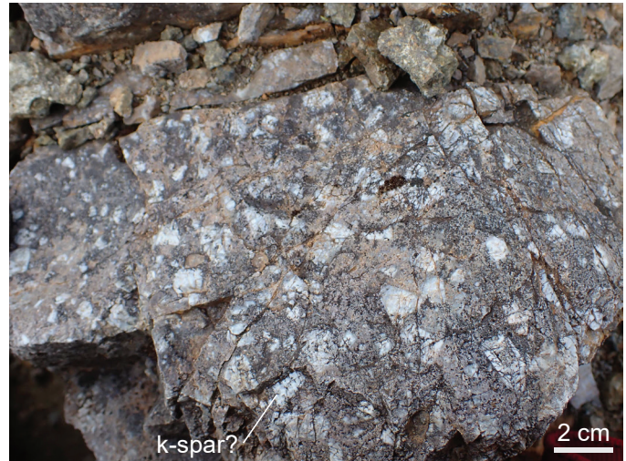
Fig. 17. Galore Creek plutonic suite syenite to monzodiorite unit (LTrGdm) from near the Grizzly occurrence. Iron carbonate-altered, feldspar porphyritic syenite-monzonite with 20-30% tabular, pale potassium(?) feldspar.
