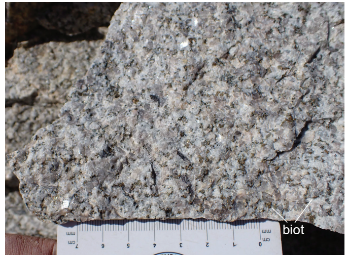
Fig. 22. Cone Mountain plutonic suite granodiorite unit (EJCgd) from Navo pluton. Medium-grained, equigranular to weakly potassium feldspar megacrystic, biotite-granodiorite with 15% K-feldspar megacrysts.
