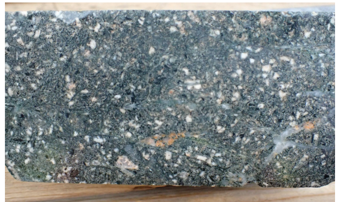
Fig. 9. Stikine plutonic suite granodiorite to quartz monzodiorite unit (LTrSgd) at the Schaft Creek deposit; porphyry to crowded porphyry with 20-50% feldspar.
