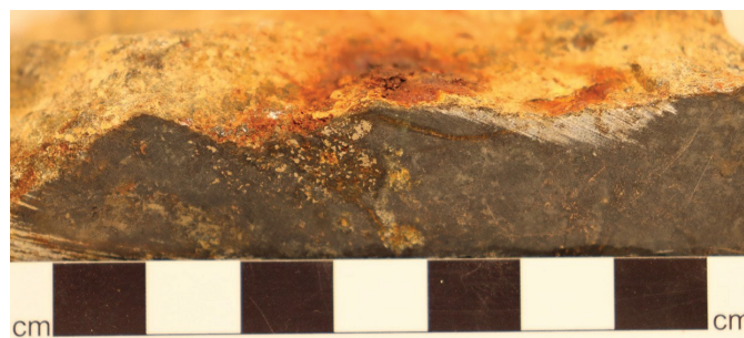
Fig. 5. Cut sample MMI06-36-3 biotite hornfels showing rusty weathering exterior and dark brown-grey interior. Biotite was extracted from this sample for ^{40}\text{Ar}/^{39}\text{Ar} analysis.
