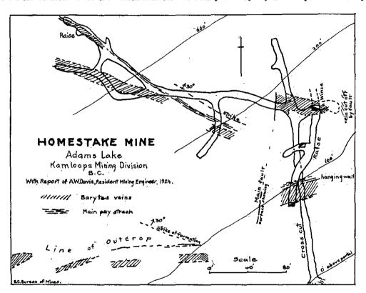
200 feet. This ore consists of a replacement of the schist, there being a central seam of high-grade silver-bearing material with the wall-rock on each side of it carrying lower values in silver. As an example of the values, the results are given of the samples taken in the crosscut to the south of the main drift, where the vein was cut. These are as follows:—
