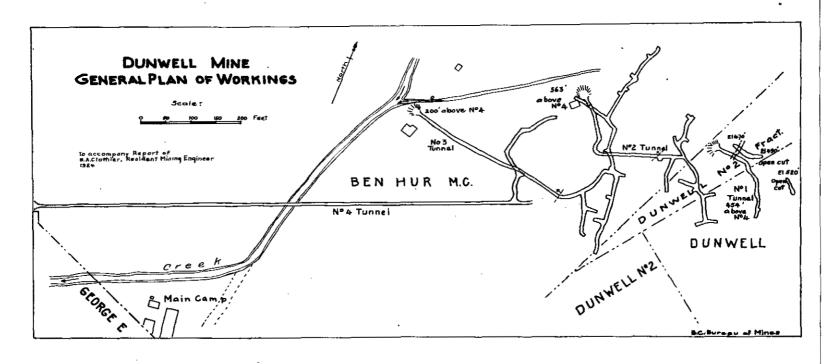
a drift was driven north on the foot-wall vein a distance of 150 feet, encountering patches of ore, but nothing of importance. A crosscut had been driven 90 feet east when the work closed down without encountering the *Dunwell* vein, though it must be very close to it.
