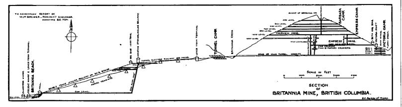
in the older sections presented a condition that necessitated the forming of a new transportation in order to deliver preliminary crushed ore to bins on the 2,200-foot haulage-level on the opposite side of Britannia mountain and necessitated the extension of the main haulage-tunnel.
