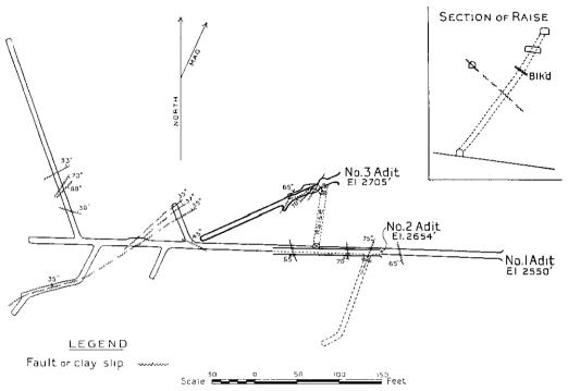
Red Buck Mines, Ltd. Plan of principal workings after company surveys.
