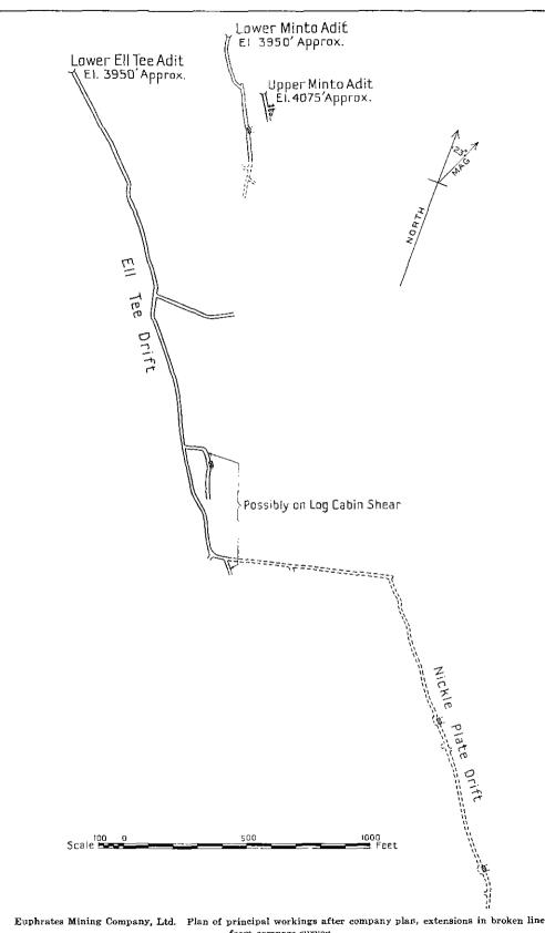
Euphrates Mining Company, Ltd. Plan of principal workings after company plan, extensions in broken lines from compass survey.
