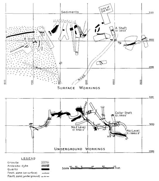
Golden Zone Mines, Ltd. Plan of principal, surface, and underground workings after surveys by company.
