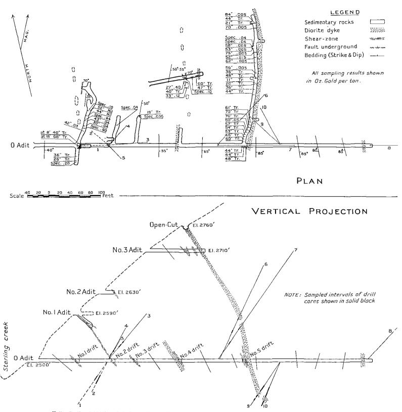
Hedley Storling Gold Mines, Ltd., Patsy No. 2 workings. Plan and vertical projection on line of "O" adit, from compass survey.
