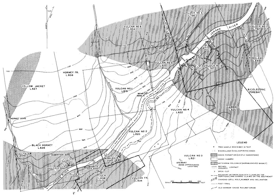
FIG.10. SUNLOCH - GABBRO, PLAN SHOWING GEOLOGY, MINERALIZED ZONES AND WORKINGS, LOCATIONS OF TREE SAMPLES, AND SOME DIAMOND-DRILL HOL 25.
