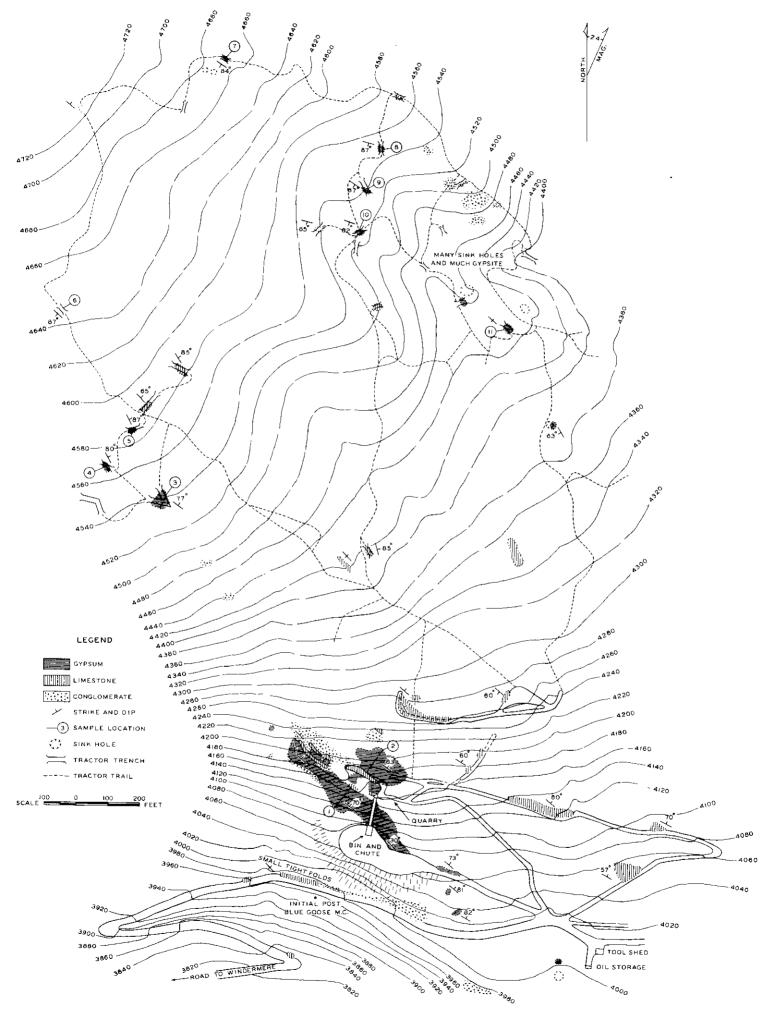
FIG.16. PLAN OF COLUMBIA GYPSUM WORKINGS.
