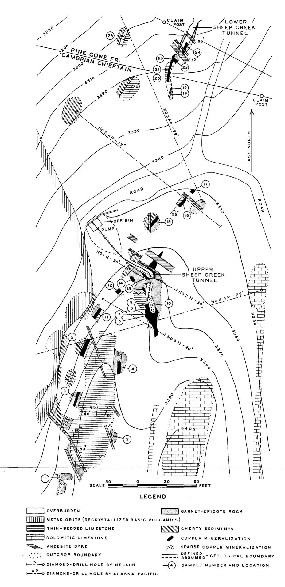
FIG.6. CAMBRIAN CHIEFTAIN-SURFACE GEOLOGY, DIAMOND-DRILL HOLES, AND WORKINGS ON MAIN SHOWINGS. At present a year-round water supply is not readily available. If the necessity arises, however, it should be possible to obtain water from one of several small lakes above and about a mile to the east and southeast of the main showing.
