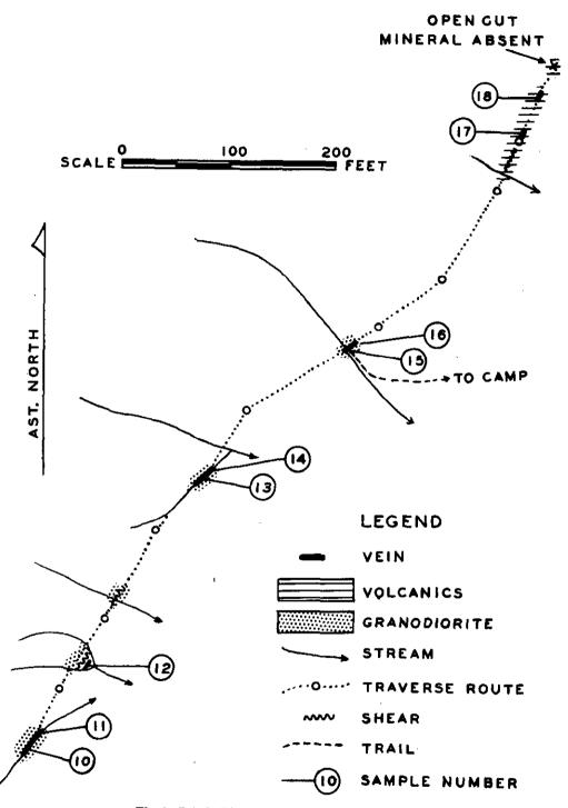
Fig. 8. Britain River-plan of upper quartz vein.
