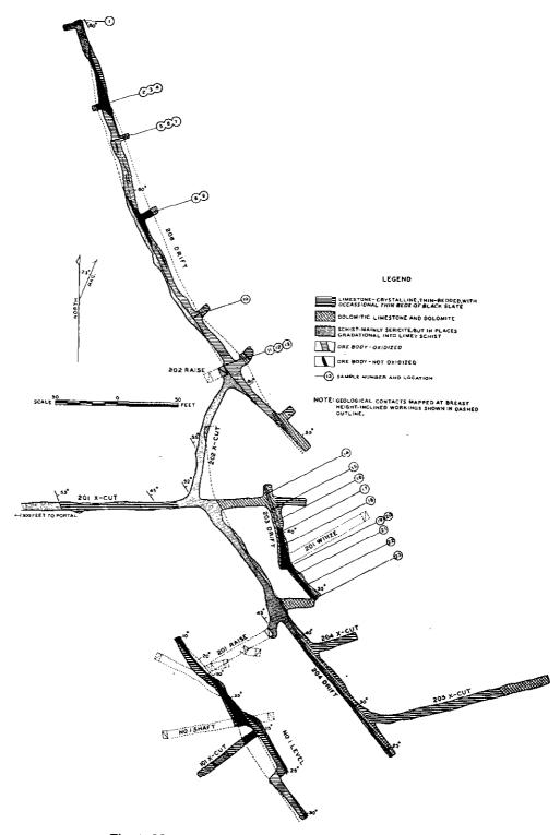
Fig. 4. Mastodon workings-geology and sample locations.
