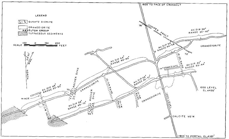
Figure 3. Western Tungsten Copper Mines Limited-plan of 1000 and 1200 levels, Rocher Deboule mine.
