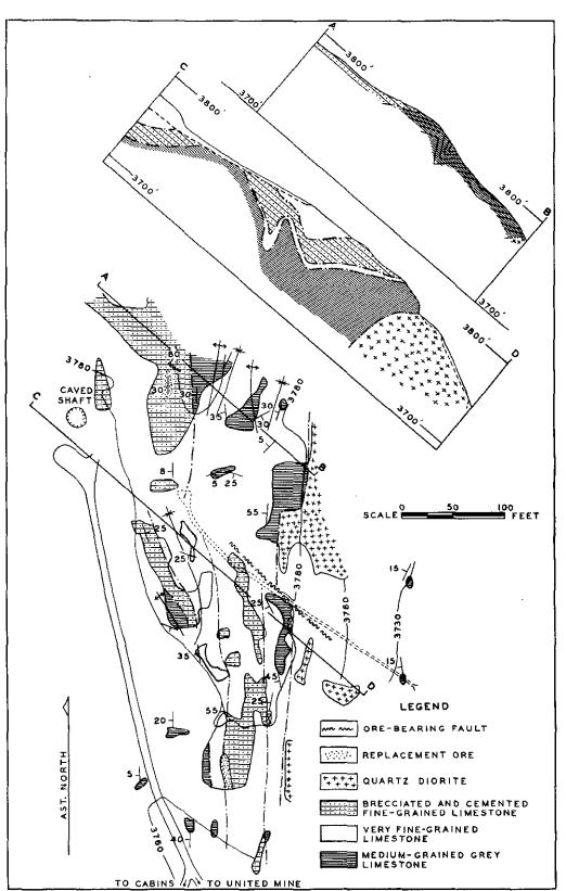
Figure 10. Geological plan and sections of Star mine.
