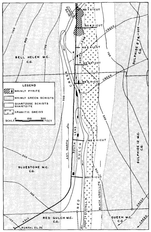
Figure 2. Ecstall River pyrite deposit-main deposit and workings.
