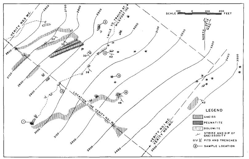
Figure 6. Tape and compass survey on Verity claims.
