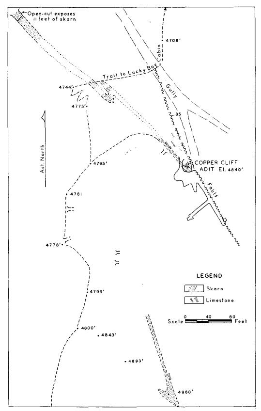
Figure 7. Major Explorations Limited-skarn exposures on the Lucky Strike claim.
