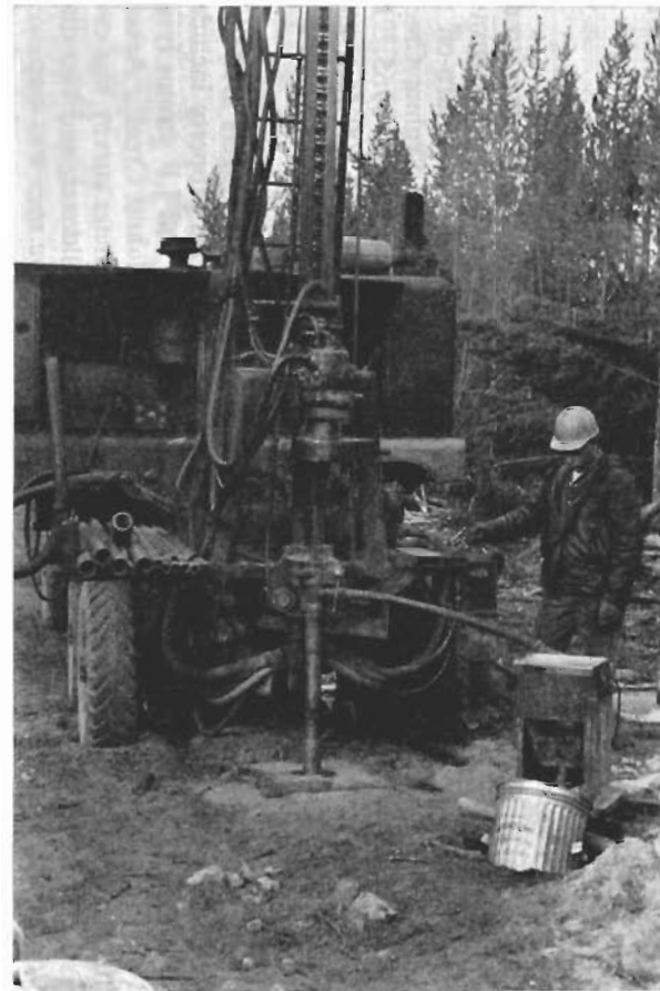
Truck-mounted percussion drill on Lornex property.
