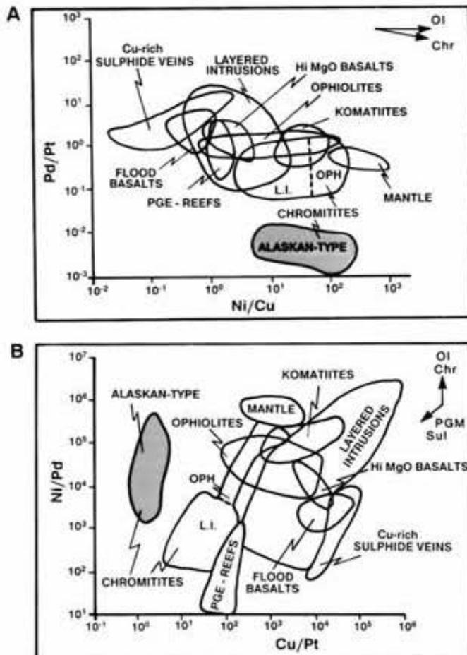
Figure 10.14. A. Pd/Pt versus Ni/Cu and B. Ni/Pd versus Cu/Pt plots for chromitites from Alaskan-type complexes (as represented by the Tulameen complex) and various mafic and ultramafic rock types, copper-rich sulphide veins and PGE reefs (after Barnes, 1990). Vectors as in Figure 10.11.
