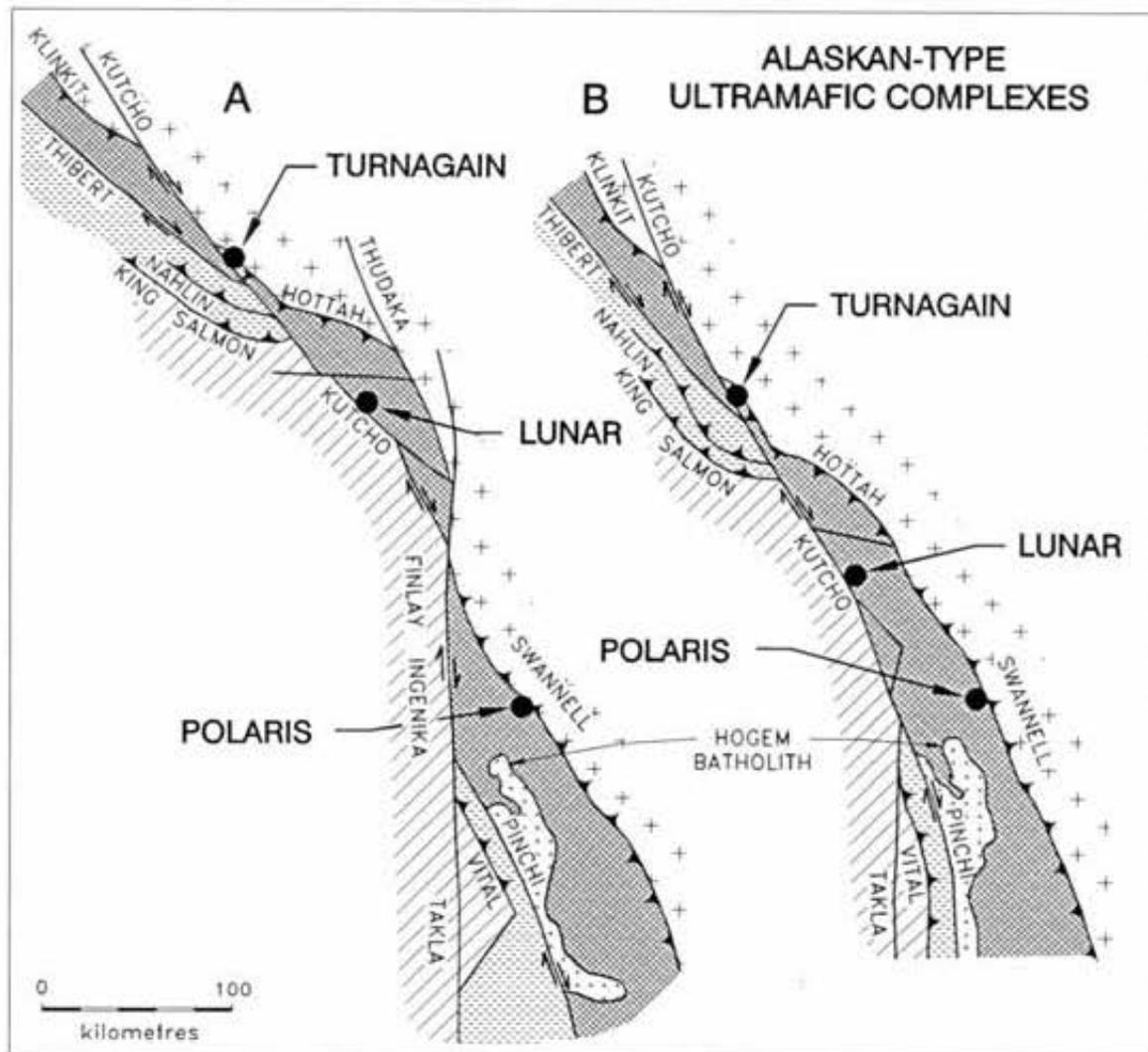
Figure 11.1 Partial restoration of Alaskan-type complexes in north-central British Columbia. A. Generalized terrane elements and major faults. B. Restoration of 60 kilometres of movement on the Thudaka fault and 50 kilometres on the Finlay and Ingenika faults (after Gabrielse, 1985). Patterns as in Figure 11.2
