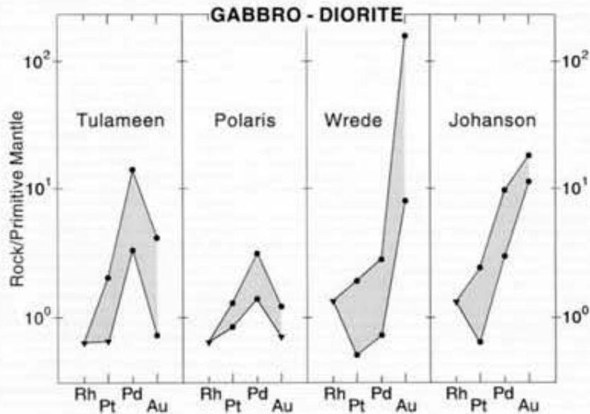
Figure 10.3. Range of mantle-normalized noble metal patterns in gabbroic to dioritic rocks of Alaskan-type complexes in British Columbia. Normalizing values and symbols as in Figure 10.1 except sulphide symbols which distinguish individual samples.
