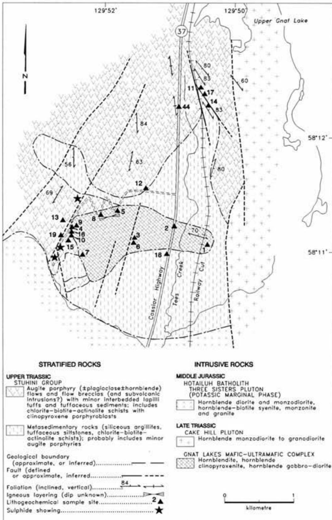
Figure 3.2. Geologic map of the Gnat Lakes mafic-ultramafic complex showing distribution of geochemical sample sites and sulphide showings.
