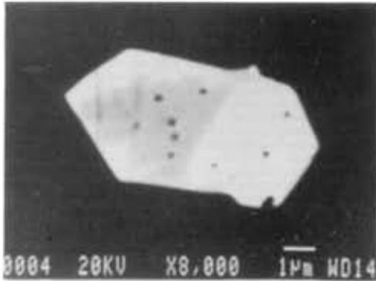
Photo 10.3. SEM image of two attached euhedral crystals of platinum alloy hosted by chromite (black) in Tulameen chromitite. Larger crystal has a core of "tetraferroplatinum" (dark grey) and rim of "isoferroplatinum" (white) in irregular contact with the core. The smaller crystal seems to consist entirely of isoferroplatinum, probably because the plane of the section traverses the rim of this crystal (*cf.* Analyses 2 and 13, Table 10.2A).
