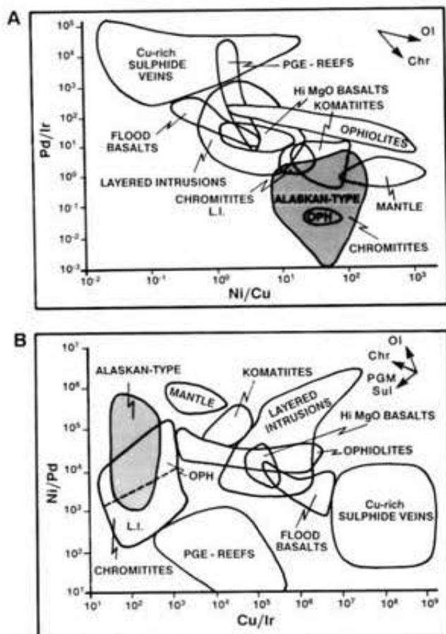
Figure 10.12. A. Pd/Ir versus Ni/Cu and B. Ni/Pd versus Cu/Ir plots for chromites from Alaskan-type complexes (as represented by the Tulameen complex) and various mafic and ultramafic rock types, copper-rich sulphide veins and PGE reefs (after Barnes, 1990). Vectors indicate addition of olivine (Ol), chromite (Chr), sulphides (Sul) and platinum-group minerals (PGM).
