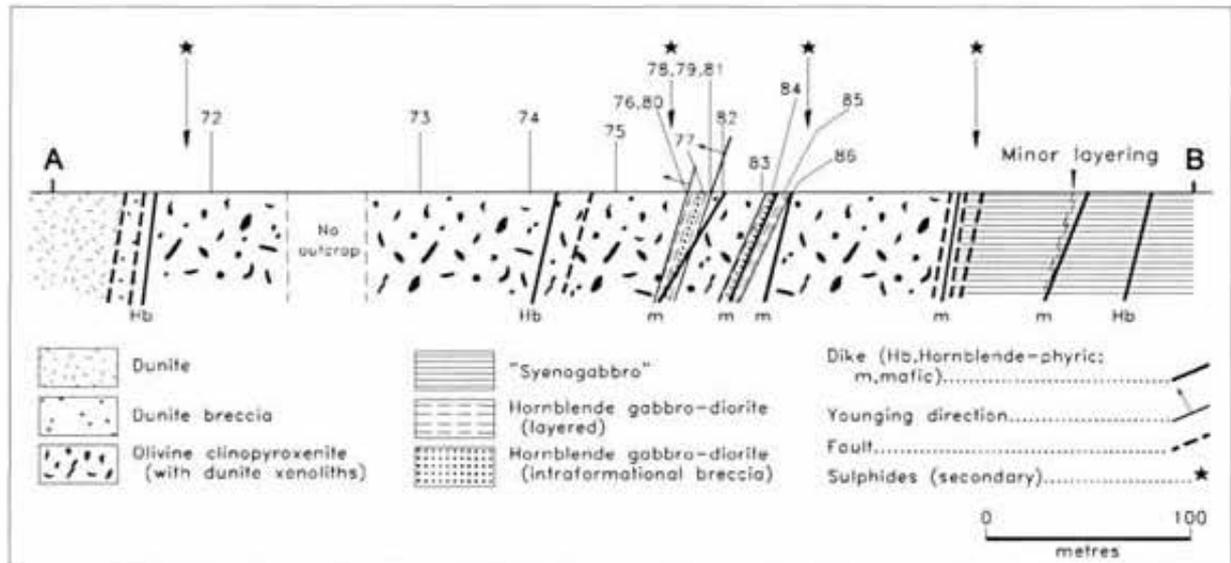
Figure 9.4. Stratigraphic section along the Tulameen River bed at the eastern margin of the dunite (see Figure 9.3 for location).
