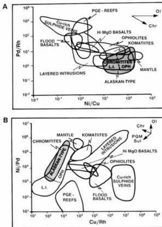
Figure 10.13. A. Pd/Rh versus Ni/Cu and B. Ni/Pd versus Cu/Rh plots for chromites from Alaskan-type complexes (as represented by the Tulameen complex) and various mafic and ultramafic rock types, copper-rich sulphide veins and PGE reefs (after Barnes, 1990). Vectors as in Figure 10.12.
