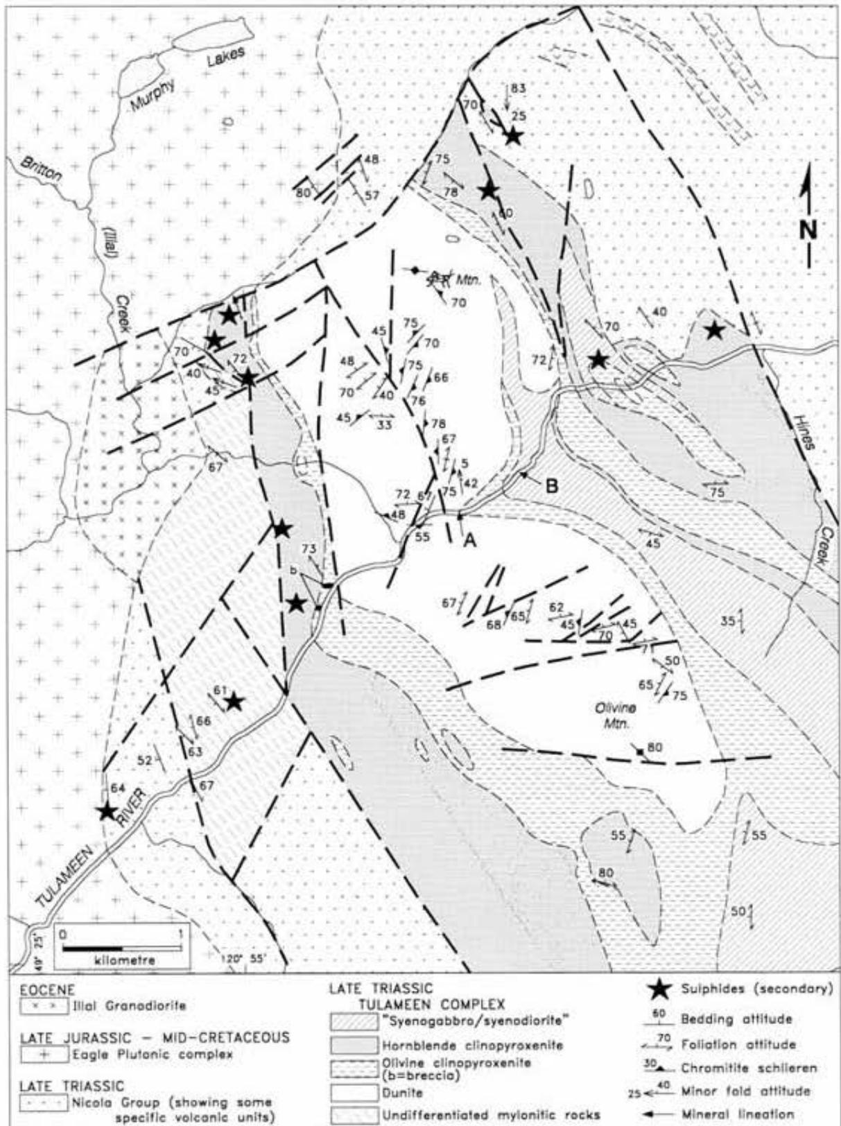
Figure 9.3. Detailed geologic map of the northern part of the Tulameen ultramafic complex (modified after Findlay, 1963 and Greig, 1989). A-B refers to the location of the measured stratigraphic section (Figure 9.4).
