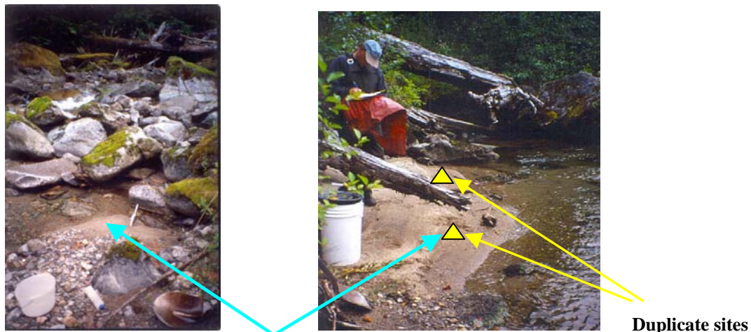
Figure 3. Stream bars with preferred sediment samples sites. A PVC pail and 1 mm stainless steel screen to wet sieve a bulk (10-12 Kg) sample for later heavy mineral separation is shown on the right.
