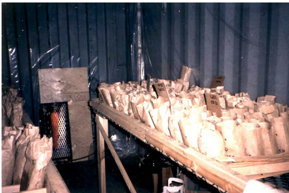
Figure 7. An example of a sediment sample drying area. Tags have been inserted between the bags identify individual sample batches.
