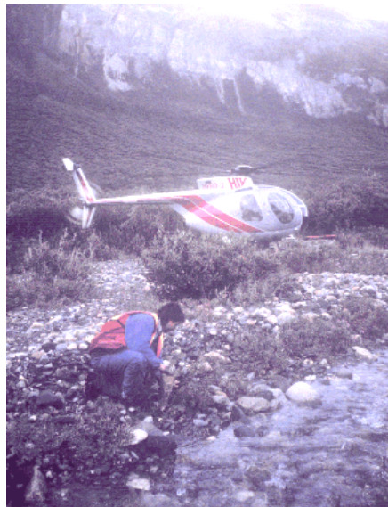
Figure 1. Helicopter supported stream sediment and water sampling. The sampler is working fast, but carefully to fill the bag with sediment from a sand-gravel bar so that the helicopter landing time is minimized. Sediment and water and data recording will typically take between 3 to 5 minutes. Commonly, the helicopter will carry a crew of two who will “leapfrog” to alternate sample sites during the traverse.
