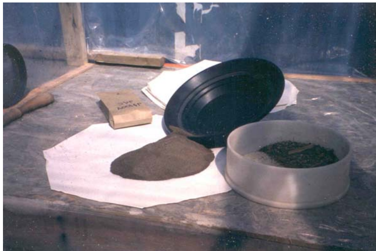
Figure 9. Processed stream sediment sample. The 1 mm nylon screen is shown on the right with a gold pan utilized to capture the < 1 mm sediment.
