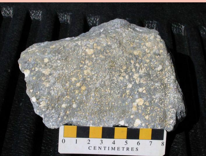
Brucite-bearing boulder from Kennedy Lake mine area. On weathered surfaces, brucite alters to white, soft, chalk-like patches consisting of
