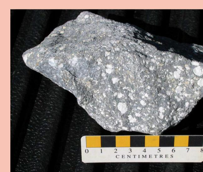
Angular brucite-bearing rock fragment, Kennedy Lake mine dump. Its presence suggests that brucite-bearing rocks may have been closely associated with magnetite ore.
