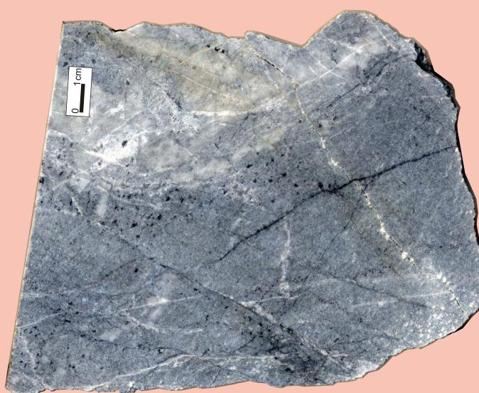
On fresh surface brucite has a greasy appearance and dark blue-gray colour. It occurs as individual, Where the fractures are open, it alters to white
