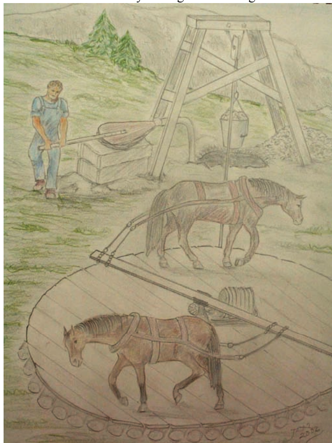
Figure 15 'Air in. Ore out' Life at the Singlehurst mine. A horse-powered winch (whim) lifts a bucket of ore from the shaft of the Singlehurst mine. Miners at the bottom of the shaft work in tunnels which follow the ore. They depend on their co-worker with a giant bellows on surface to pump fresh air into the mine down a long pipe. (Drawing by JoAnne Nelson).
