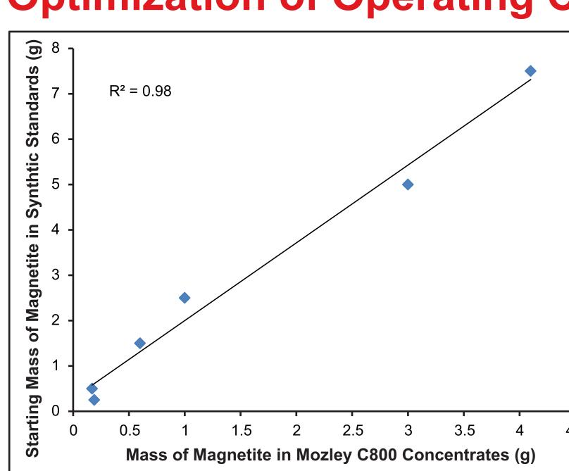
were used to test operating parameters. They were made predominantly of quartz with 0.33 to 10 wt. % each of magnetite, garnet, and fluorite. The excellent correlation  $(R^2=0.98)$  between magnetite in synthetic standards and in Mozley C800 concentrates indicates consistent concentration. Magnetite concentration increased by 5.5 to 228.2 times. From Mackay et al. 2015.
