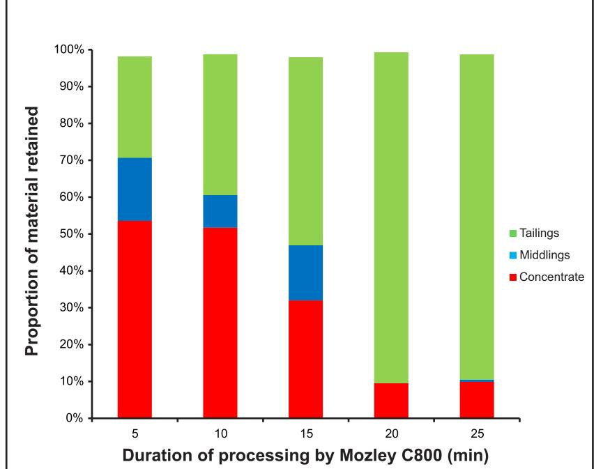
The proportion of concentrate for five identical sub-samples  $(\sim 75g)$  of AL-13-16 'decreased with increasing processing time. All other parameters 15 minute time interval time is a compromise which ensures adequate concentration of heavy minerals, minimizing loss to tailings. From Mackay
