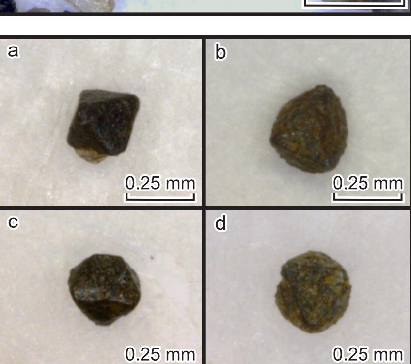
mineral concentrate (sample AL-13-16) containing apatite (Ap), pyrochlore (Pcl), columbite-(Fe) (Cmb), and magnetite (Mag). Lithic fragments (Lit), and grain aggregates (Agg) are also present. Pyrochlore is identified by its distinctive octahedral crystal habit. Optical identification can be difficult in highly weathered grains. A magnetite from columbite-(Fe) and other non-magnetic
