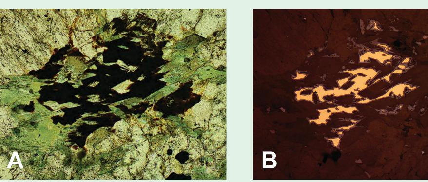
oy/intergrown with actinolite/actinolitic hornblende in hornblende clinopyroxenite (plane polarized light); B) Same view in reflected light; C) Acicular actinolite in interstitial chalcopyrite in magnetite hornblendite (note tarnished inclusion of chalcopyrite in hornblende, lower right).
