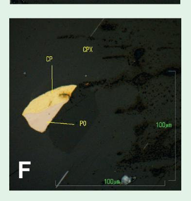
A) Swarm of chalcopyrite inclusions in intercumulus magnetite (magnetite-hornblende clinopyroxenite); B) crvstal morphology: C) Faceted inclusion of chalcopyrite-pyrrhotite netite clinopvroxenite): D) Magnetite hornblendite (plane- polarized light): rite and bornite in hornblende (circle in D) showing chalcopyrite exsolution lamellae and rim of covellite ; F) Composite inclusion of chalcopyrite-pyrrhotite in clinopyroxene (hornblende-magnetite
