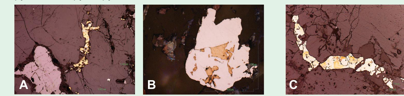
A) Pyrite (white) replacing interstitial chalcopyrite in hornblende-magnetite clinopyroxenite; B) Relict chalcopyrite in interstitial pyrite (white) in hornblende-magnetite clinopyroxenite; C) Interstitial pyrite containing ghost remnants of chalcopyrite in hornblende-magnetite clinopyroxenite.
