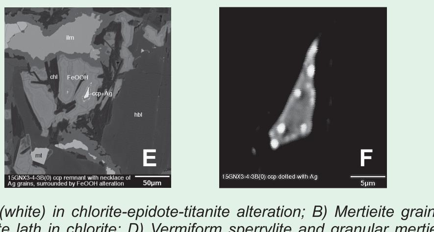
SEM images: A) Fine-grained mertieite (white) in chlorite-epidote-titanite alteration; B) Mertieite grain in chlorite-goethite assemblage; C) Mertieite lath in chlorite; D) Vermiform sperrylite and granular mertieite grains in chlorite and Cu-silicate; E) Remnant grain of interstitial chalcopyrite in chlorite-Fe-hydroxide (magnetite hornblendite); F) Chalcopyrite grain in E showing necklace of Ag mineral (white dots).
