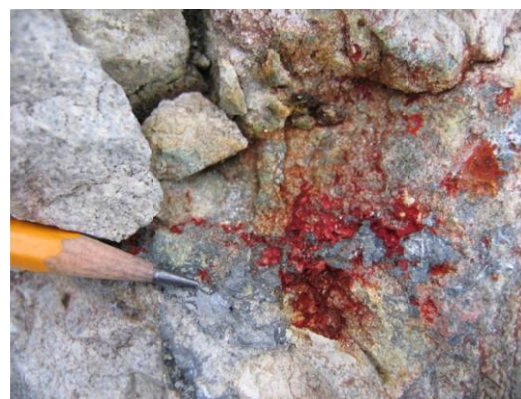
Figure 5. Typical bright red stain caused by reaction of "Zinc Zap" solution with zinc-rich mineralization, east-central British Columbia.
