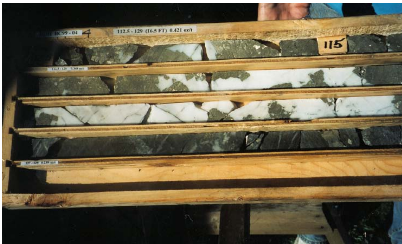
Photo 5. Drill-core intersection of the BC vein, showing coarse-grained pyrite in a gangue of white quartz.
