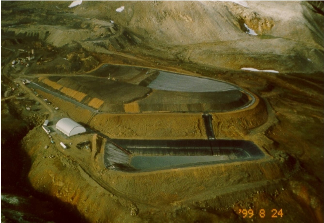
Figure 6. Totem heap leach-pad being loaded with Ursa ore (dark coloured) and Kodiak A ore (light coloured). The pond in the foreground is for drainage control from storm events.
