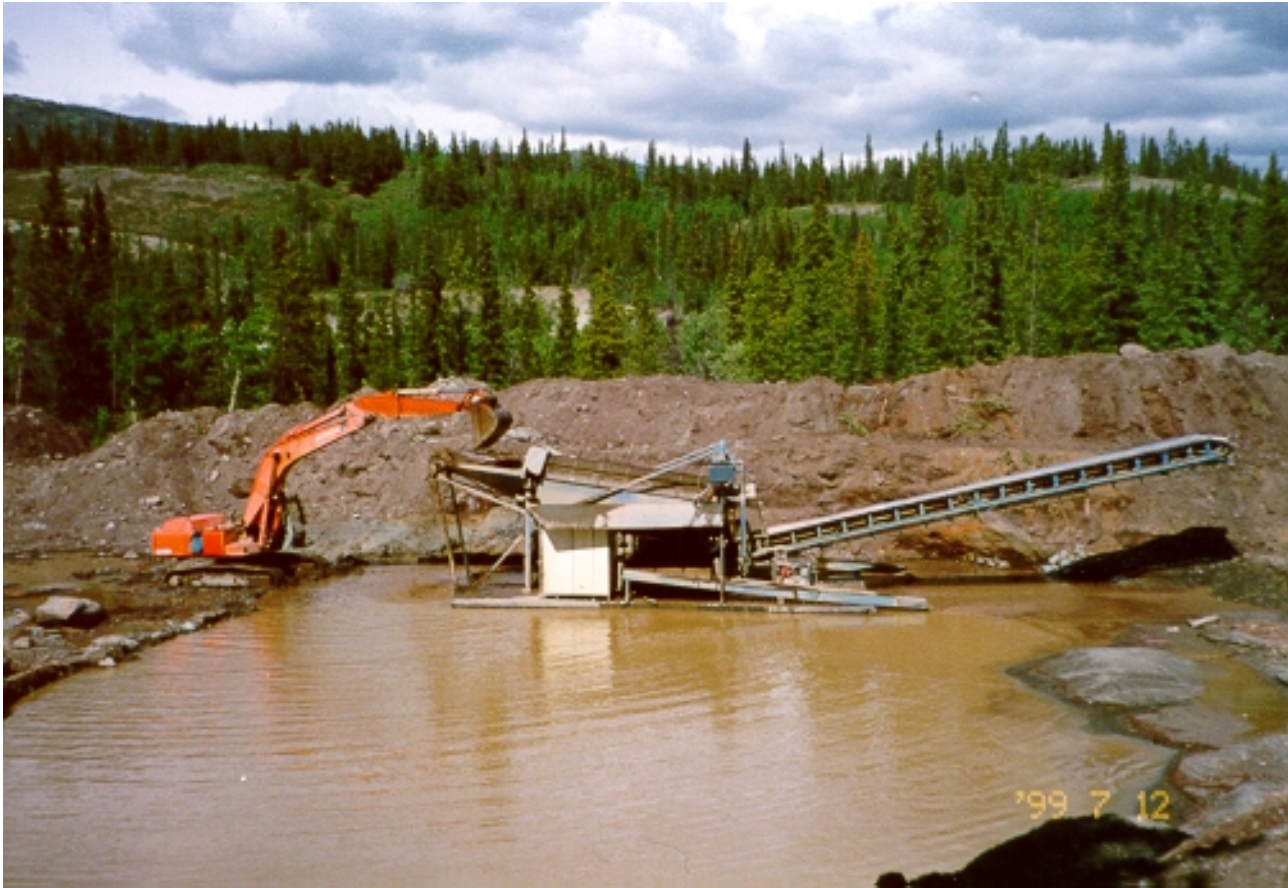
Figure 7. “New Zealand” style floating wash plant, fed by an excavator, at Kim Ferguson’s placer mine on Pine Creek.
