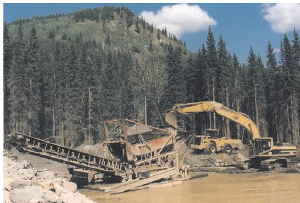
Photo 13. Mobile processing plant in use on Manson Creek, Angel Jade Mining.
