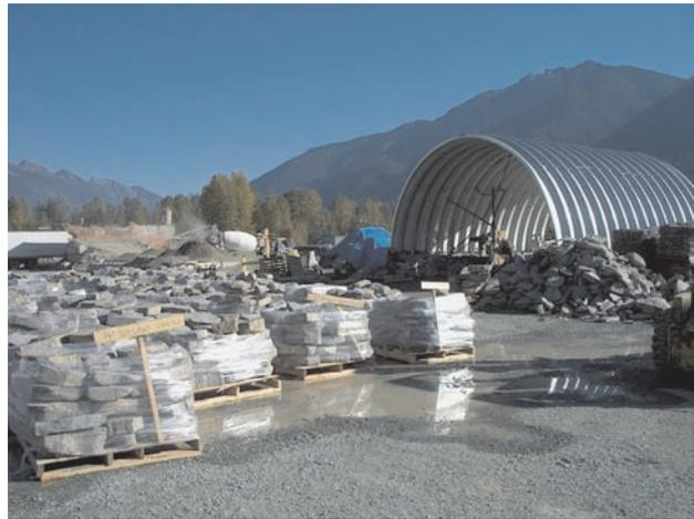
Photo 2. Palletized basalt column segments and gang saw at Mountain High Properties Inc.'s dimension stone plant, Pemberton.
