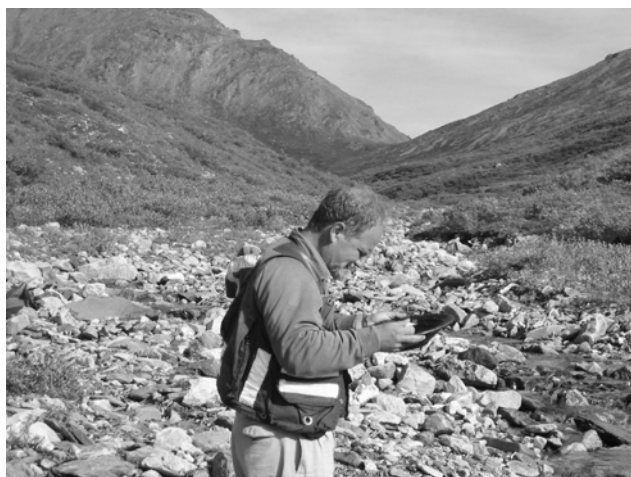
Photo 8. George Simandl, B.C. Geological and Development Branch, examines heavy mineral concentrate for diamond indicator minerals on the Xeno property.
