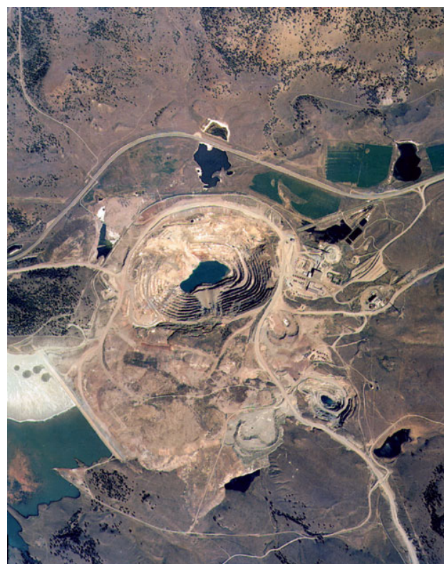
Figure 4-12. Aerial view of the Afton mine complex with the Afton pit in the centre with mill/office buildings to the east (right) and the Pothook pit to the southeast. The Afton main zone extends in a southwesterly direction from the bottom of the pit towards the tailings pond in the lower left. The Trans-Canada Highway curves around the north side of the pit. (Courtesy DRC Resources Corp)
