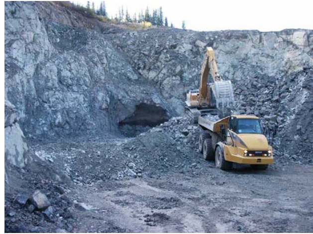
Figure 3-5. Stripping waste rock from the Creek zone open cut, Shasta gold-silver mine.
