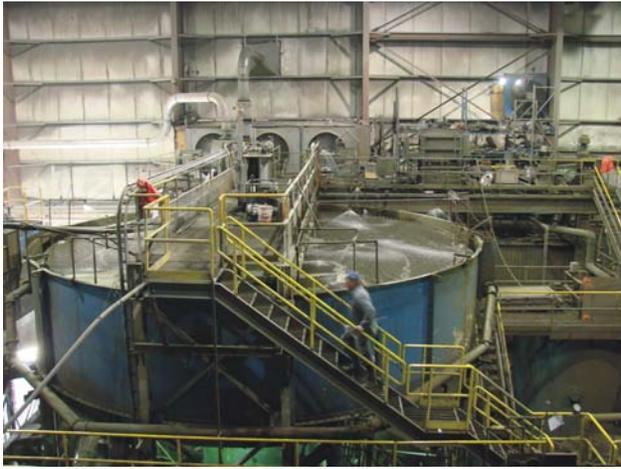
Figure 3.4. Filtration tank, Mount Polley Mine Mill.
