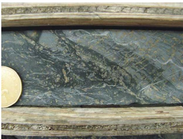
Figure 3.11. Drill core grading 33 g Au/tonne, Main Zone, Spanish Mountain.
