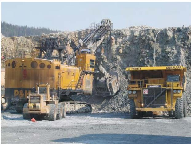
Figure 3.6. Loading operations in Granite Pit, Gibraltar Mine.
