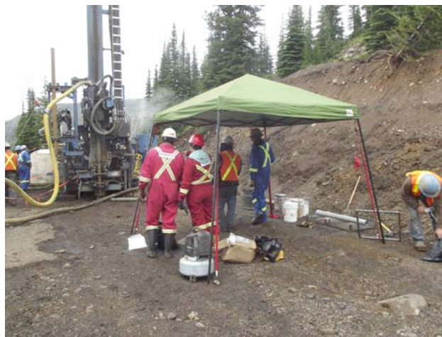
Figure 6.10. Exploration drilling on the Crown Mountain coal property (Jameson Resources Limited). Photo by Geraldine FitzGerald.
