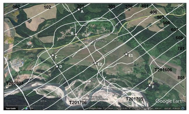
Figure 11. Location map of AEM lines flown over the study area and proposed drill targets (A-F). The erratic flight paths along some lines were necessary to avoid developed areas. Note that the density of flight lines in the study area is approximately double that in the regional survey.
