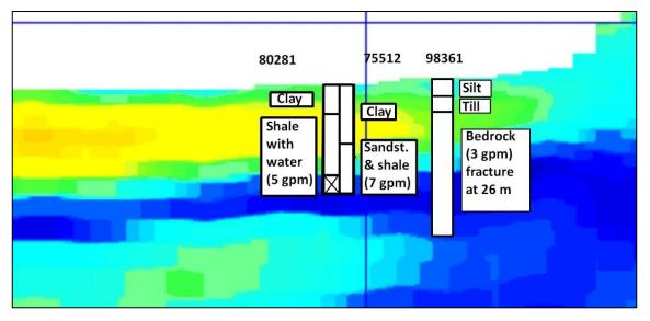
Figure 10. Lithologic logs for water wells 80281, 75512 and 98361 plotted on EM Line 118001.
