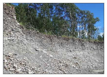
Figure 3. Alluvial terrace gravels several kilometres west of the HRFN community. The gravels are pebble to cobble sized, mostly dry and moderately well stratified.
