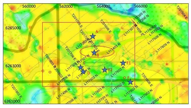
Figure 6. Location of EM flight lines overlain on the 10-15 m EM depth slice. The red circle outlines the area of the HRFN community and the red box outlines the primary study area. UTM easting and northing coordinates are shown on the top and left sides of the figure, respectively. Stars show target water well locations A to F.
