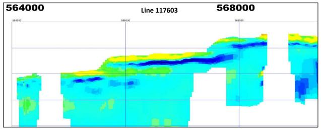
Figure 13. Northeast-trending EM sections in the central part of the study area: Upland areas and high glaciofluvial benches east of the HRFN community are shown on the right side of the figure; view towards the northwest; vertical scale on all sections is about 1:5000 (2 cm = 100 m); horizontal scales shown
