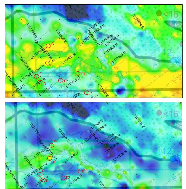
Figure 17. EM resistivity depth slices in the study area (top: 20-30 m; bottom 30-40 m) area and proposed drill targets (A-F)
