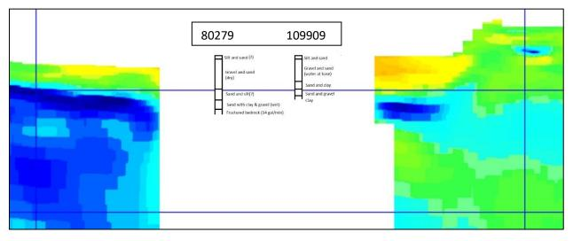
Figure 7. Lithology logs for water wells 80279 (left) and 109909 (right) plotted on EM cross-section L117202N.
