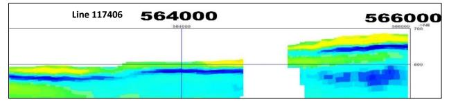
Figure 12. Northeast-trending EM sections in the northwest part of the study area: High bench northeast of the HRFN community is shown on the right side of each figure; view towards the northwest; vertical scale on all figures is about 1:5000 (2 cm = 100 m); horizontal scales shown.
