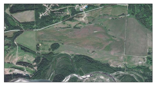
Figure 2. Air photo image of HRFN study area showing the community at the top of the figure and the Halfway River at the bottom (2017, Google Maps image). Note the abandoned channels, point bars and scroll bars along the Halfway River and remnant channel scars and longitudinal bars on the alluvial terraces south of the community
