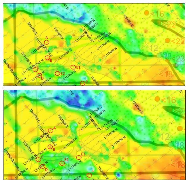
Figure 16. EM resistivity depth slices in the study area (top: 10-15 m; bottom 15-20 m) area and proposed drill targets (A-F)
