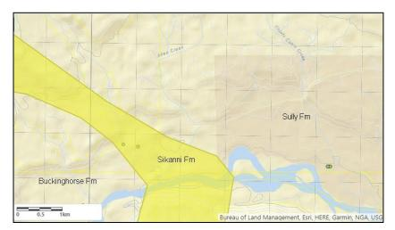
Figure 4. Bedrock geology of the study region. Dots are water wells in the BC WELLS database. Note that the two wells overlying the Sikanni Formation both produced water while those over the Sully formation were all dry.
