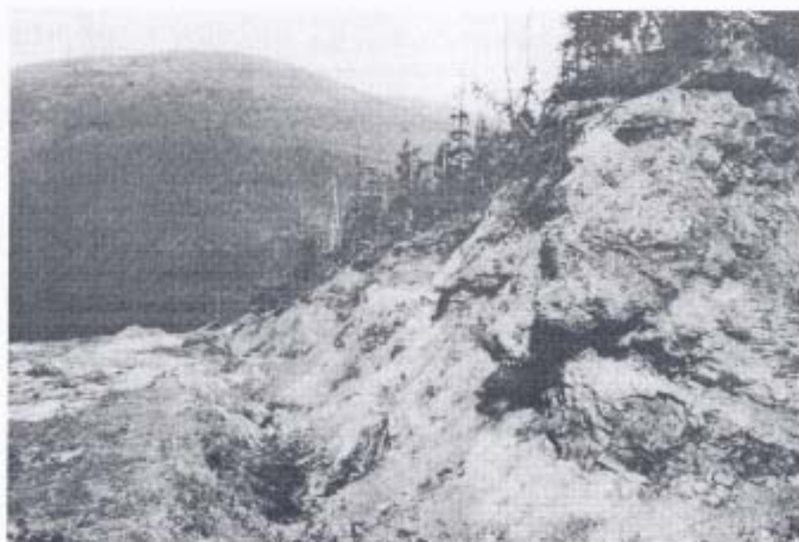
Photo 2. Midway - trench on Discovery zone. Light band is weathered massive sulphide.
